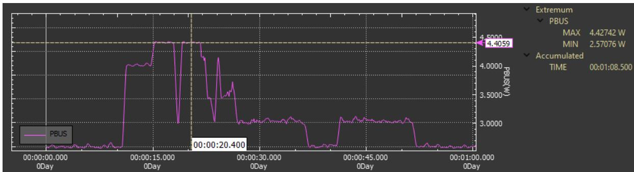
**Figure 5.8:** Power Consumption When Decompressing Stress Test Container
