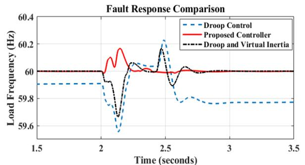
FIGURE 6. Frequency response comparison between controllers.
