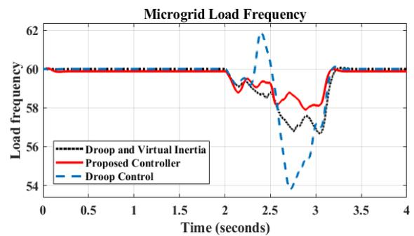
FIGURE 5. Frequency response comparison in different control systems.
