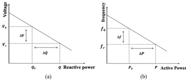
FIGURE 3. (a) P-f droop control, (b) Q-V droop control.
