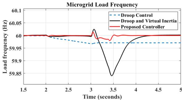
**FIGURE 7. Frequency response comparison between controller's sudden change in irradiance.**
