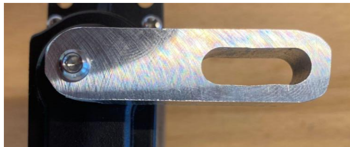
Figure 4.3: Machines slots with hand sanded rounded corners.
