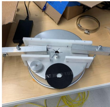
Figure 4.4: Machined Delrin plastic parts for sample storage system
