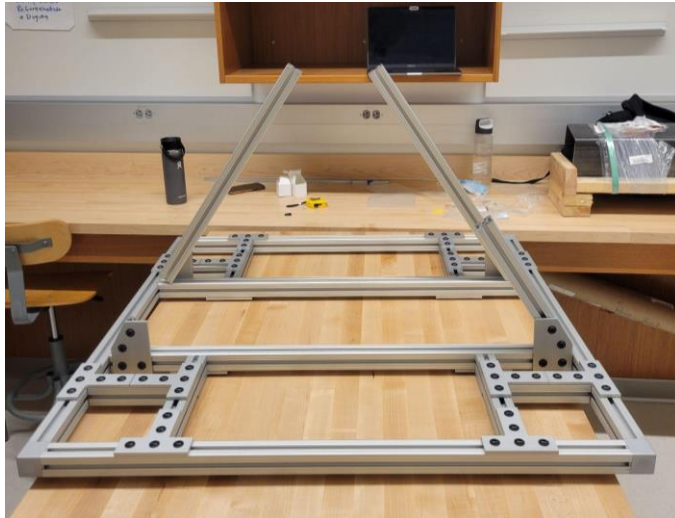
Figure 4.1: Assembled Base of Frame
