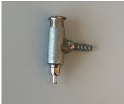
Figure 15. Coaxial needle used to create 1 mm alginate capsules.
