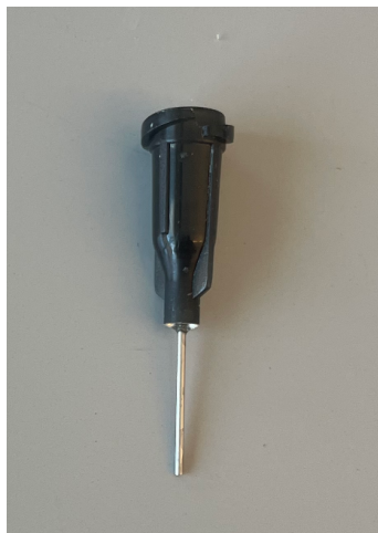
Figure 16. Standard needle used to create 3 mm alginate capsules.
