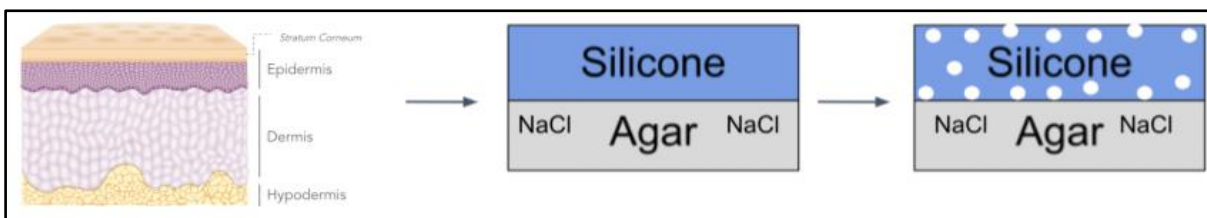
Figure 3.2: Skin phantom assembly with porous silicone and 4% agar with NaCl.
