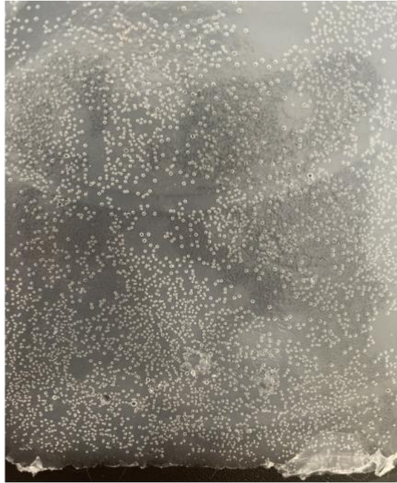
Figure 5.3: Porous silicone gel made with 1 g sugar in 15 mL silicone.
