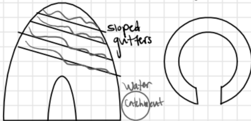
Figure D-14: Sloped Gutter Design
