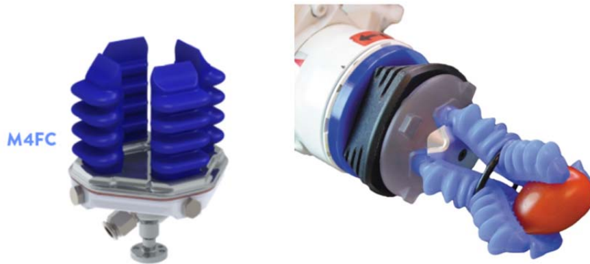
Figure 1a and 1b: Images of currently utilized soft robotic grippers in the industry [Soft Robotics; Shen, Helen]
