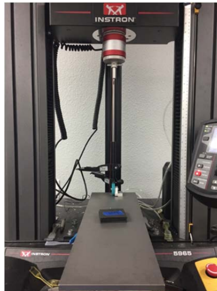
Figure 9: Instron testing apparatus for coefficient of friction testing
