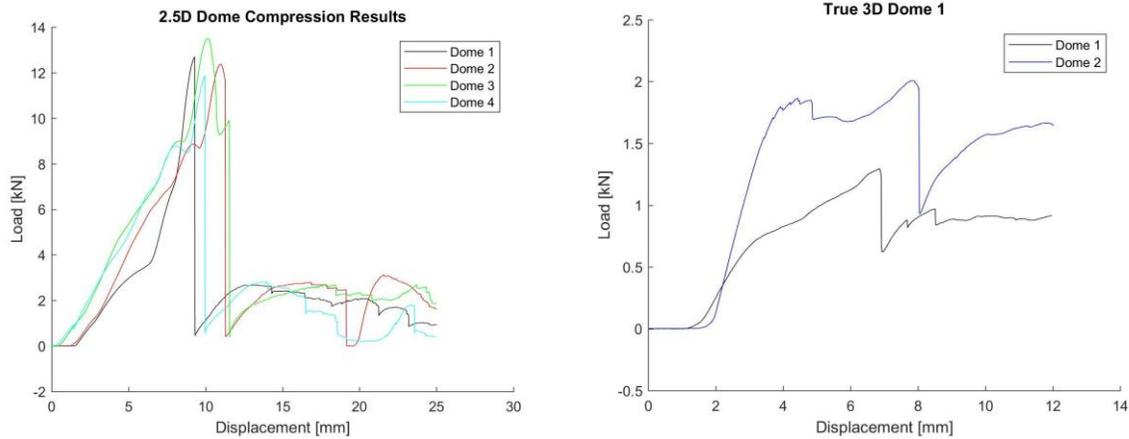
**Figure 8:** Graphical results from testing four 2.5D printed domes and two true 3D domes. The 2.5D domes experience a significant fast fracture and do not regain any strength while the true 3D domes retain their strength.
