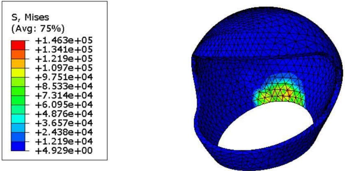
**Figure 16:** Point force Von Mises stress results, showing a max stress of 146 MPa, and an average of 12 MPa at the point of force
