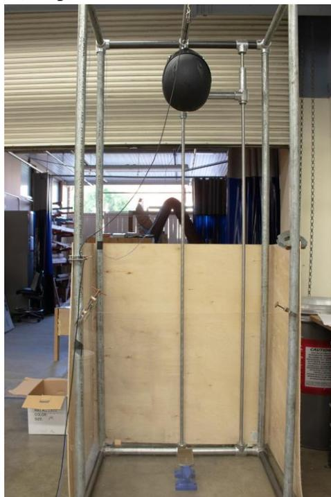
**Figure 13:** Picture of the complete test structure with the helmet mounted on the head-form, the safety guard installed, and the anvil placed at the bottom of the structure.
