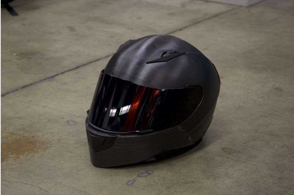
**Figure 4:** Fully assembled carbon fiber reinforced polymer 2.5D printed motorcycle helmet.
