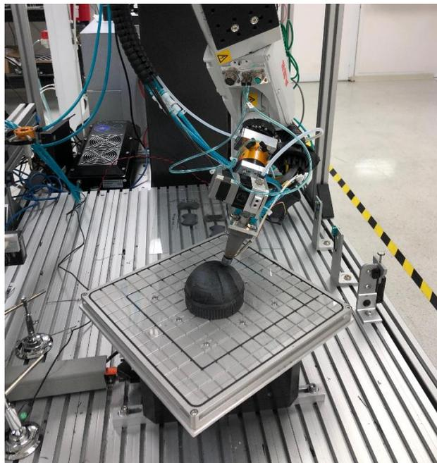
**Figure 2:** Multi-Axis Arm for 3D printing
