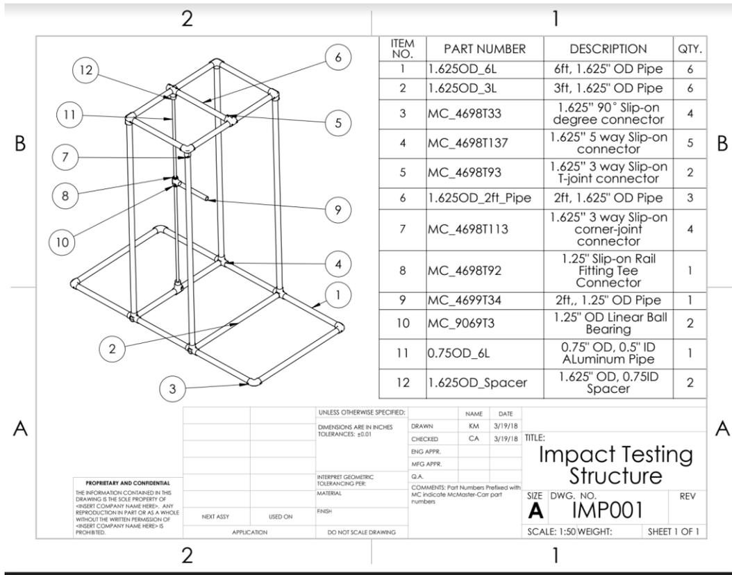
**Figure 11:** Drawing of first version of impact testing structure. This version of the structure is a monorail system.
