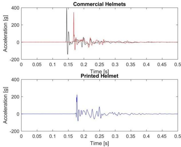
**Figure 18:** Results from the impact testing on two commercial helmets and the 3D printed helmet. The acceleration on the head form experienced between 340 and 396 g’s during the commercial helmet testing and less than 230 g’s for the 3D printed helmet.
