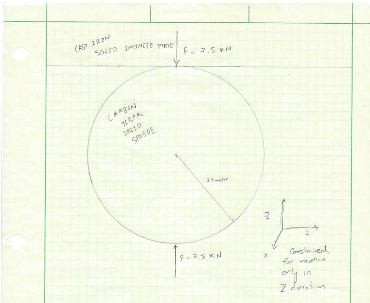
**Figure F1:** Free body diagram showing the carbon fiber sphere in contact with the cast iron plate for simplified hand calculation of maximum achieved stress.
