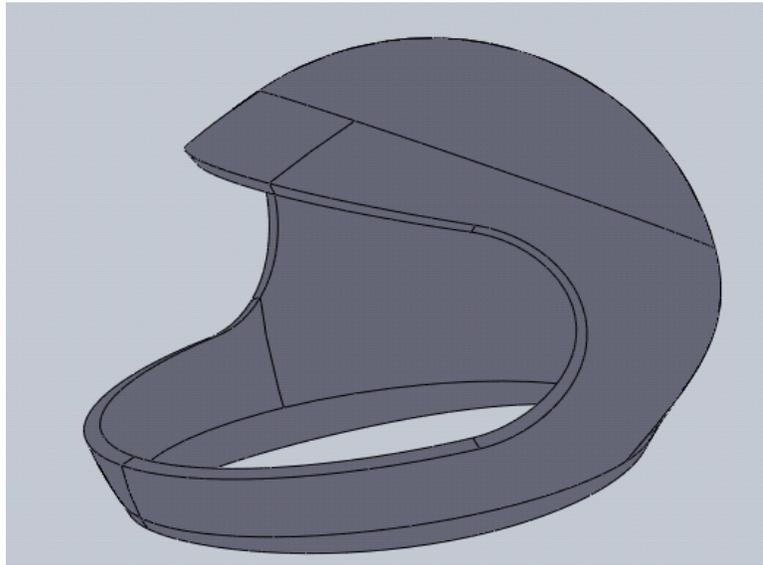
**Figure F4:** Simplified helmet used for the FEA modeling
