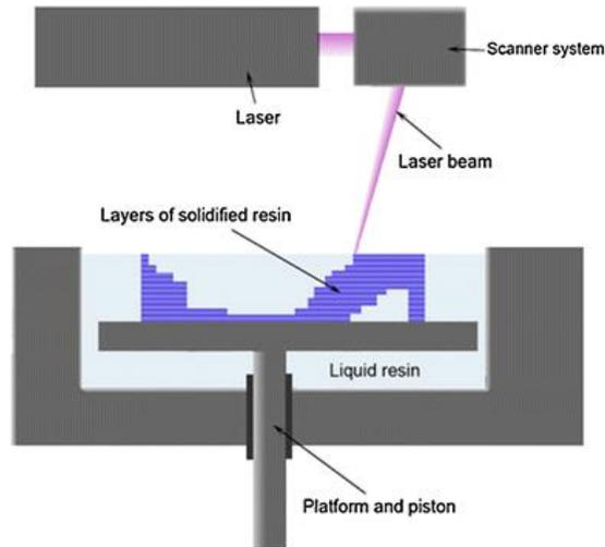
**Figure 1:** Layer method for 3D printing
