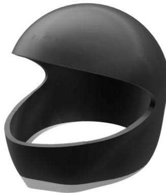
**Figure 14:** Initial CAD design of reinforced carbon fiber PEEK helmet using SolidWorks
