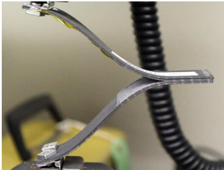
**Figure 7:** The material specimen is loaded into the Instron testing machine and displaced at the hinges until fracture. This sample pictured has delaminated approximately 30 mm.
