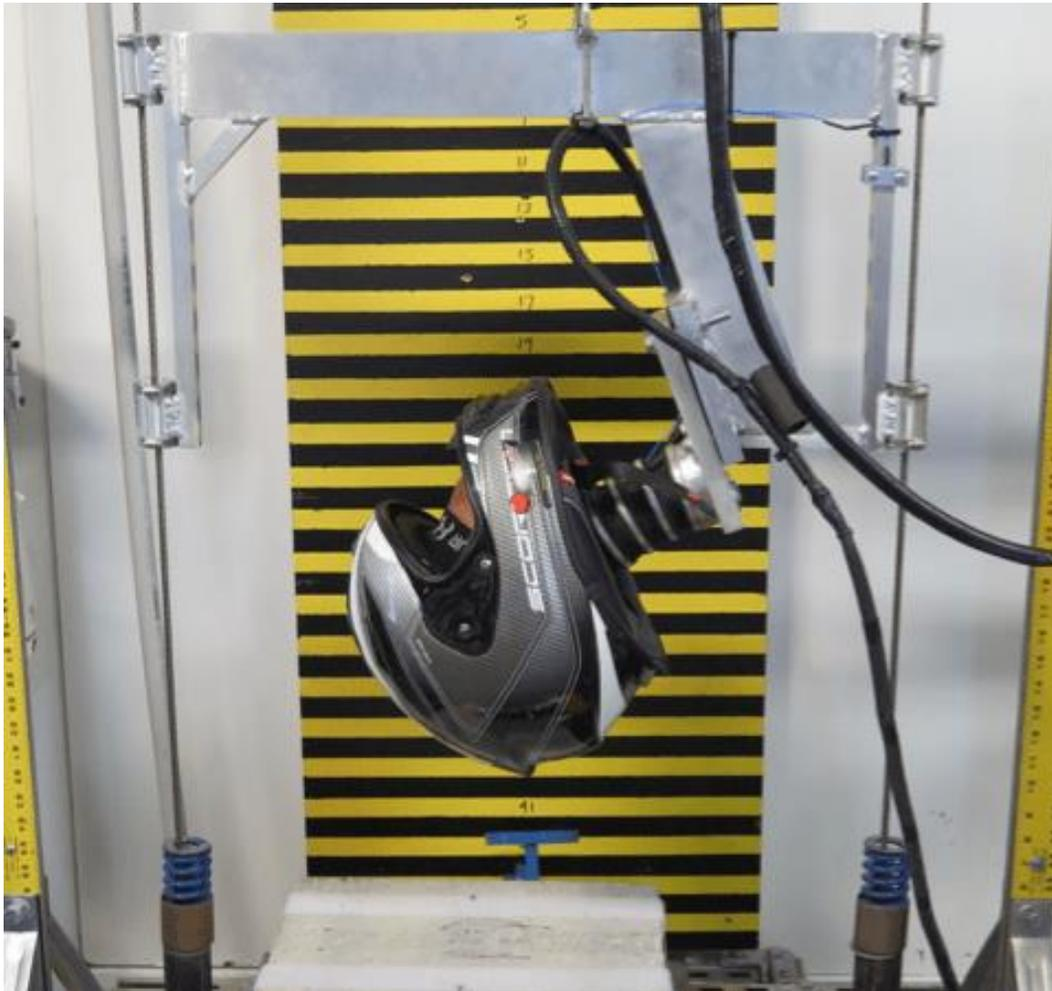
**Figure 10:** Example of a 3rd party impact test in which the helmet on a head form is dropped in a controlled fall onto a flat anvil. [6]
