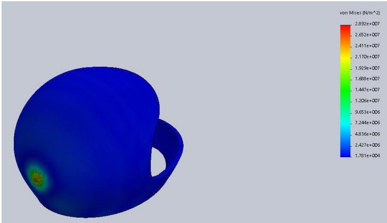
**Figure 17:** shows the results of the drop test in SolidWorks with a maximum Von Mises of 29 MPa
