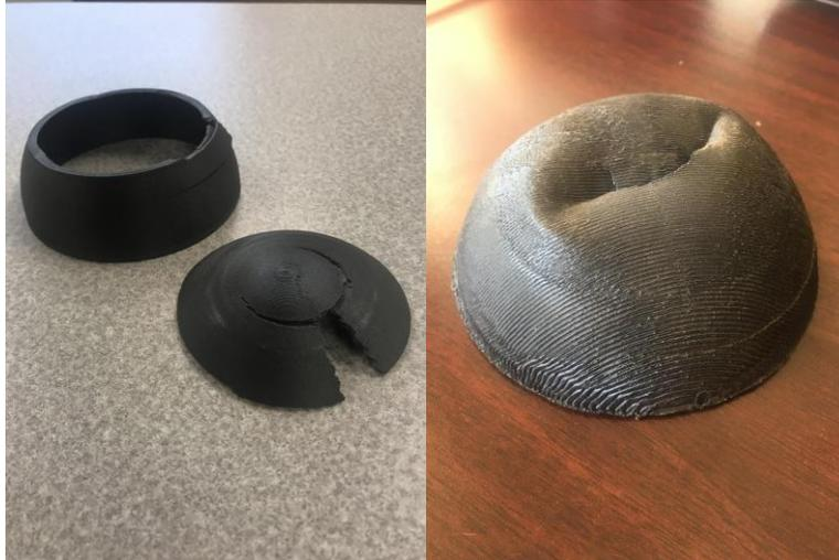
**Figure 9:** 2.5D (left) and true 3D (right) domes after compression testing. The 2.5D domes experience catastrophic failure along the printed slip planes while the true 3D domes do not have these slip planes and experience a conventional compression failure mode.
