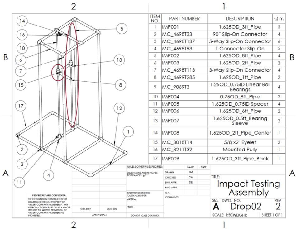
**Figure 12:** Drawing of the revision of impact testing structure. The major change is the addition of second pole (large red circle) to prevent the rotation of the head form shaft (small red circle).
