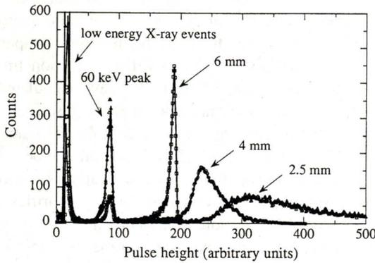
FIG. 2. Superimposed pulse-height spectra obtained with quasiparticle trapping thermistor for collimated alpha source located at 6, 4, and 2.5 mm from the thermistor edge.
