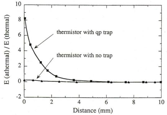
FIG. 3. Ratio of athermal to thermal phonon energy detected in each thermistor for various alpha source positions (measured relative to the respective thermistor edges).
