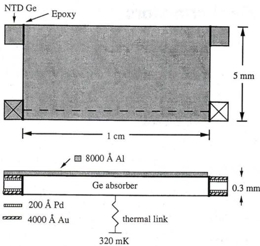
FIG. 1. Schematic diagram of the SLAPS device showing top and side views (not to scale). The two thermistors studied in this experiment are each denoted by X, and the axis scanned by the  $^{241}\text{Am}$  alpha source is indicated by the dashed line.
