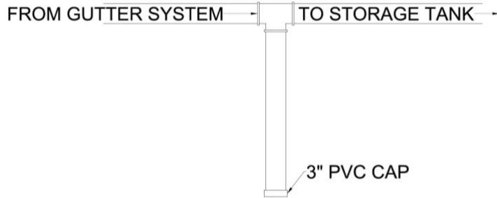
Figure 9: First flush system design.
