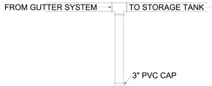
Figure 9: First flush system design.
