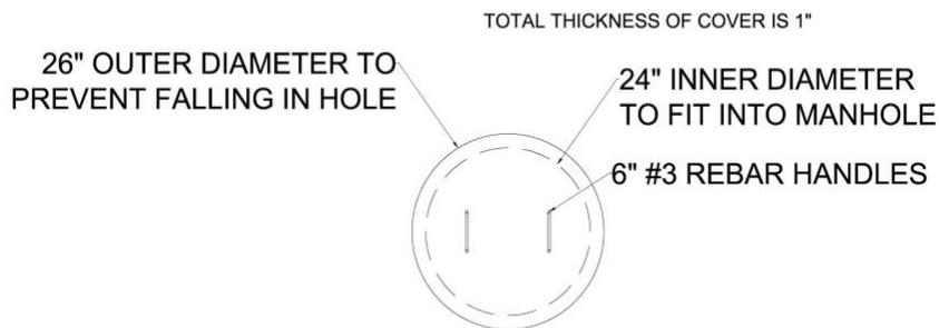
Figure 7: Manhole cover detail.
