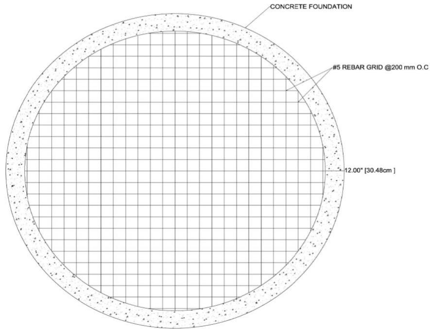
Figure 6: Rebar grid layout.
