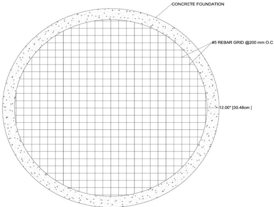
Figure 6: Rebar grid layout.
