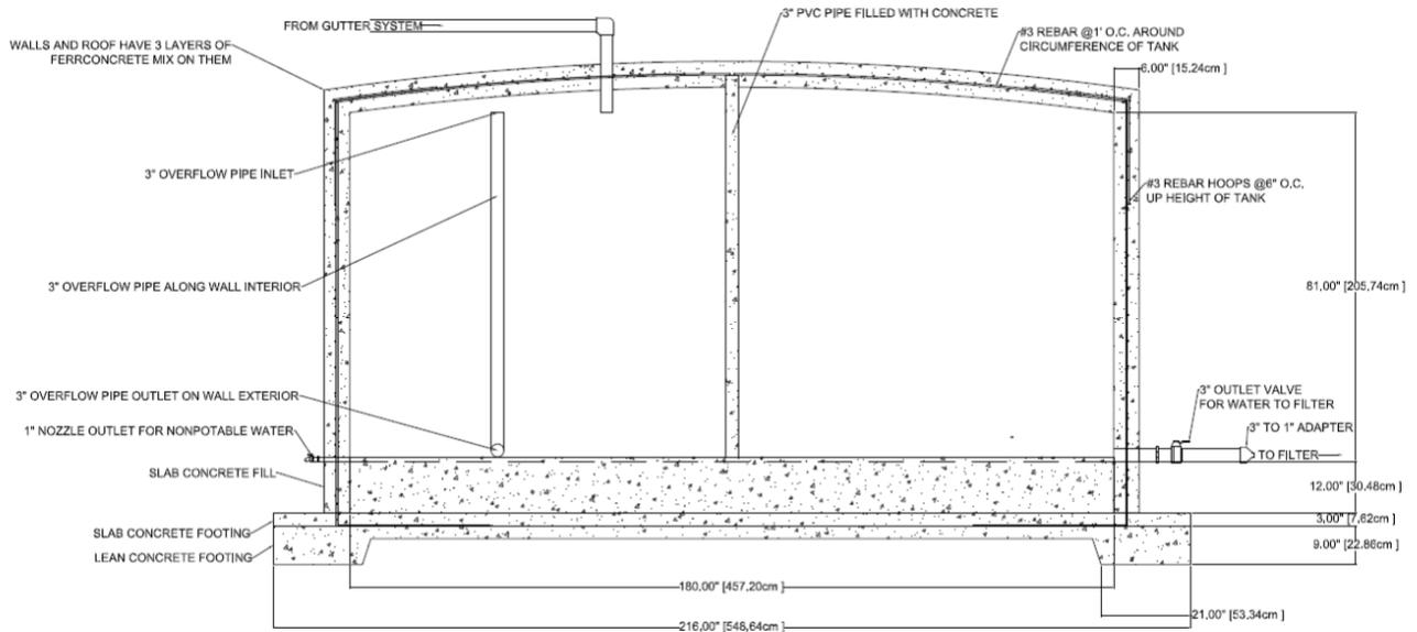
Figure 5: Cross-section of ferrocement tank design.
