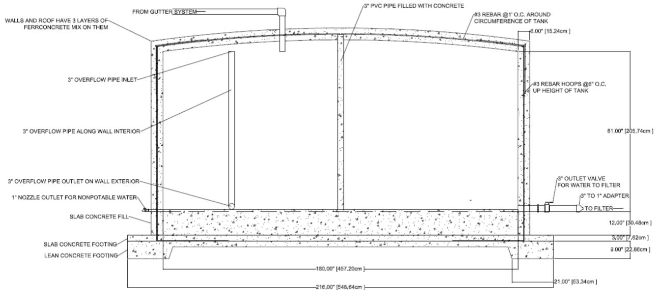
Figure 5: Cross-section of ferrocement tank design.
