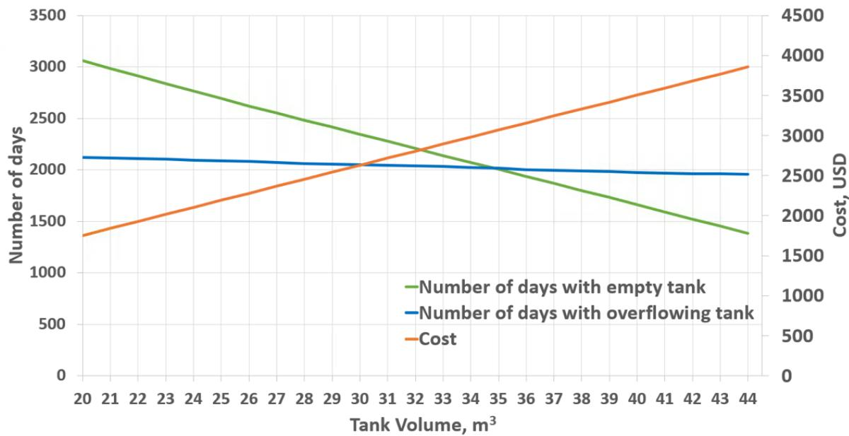
Figure 4: Cost of water storage tank sizes compared with the amount of empty and overflowing days for the tank.
