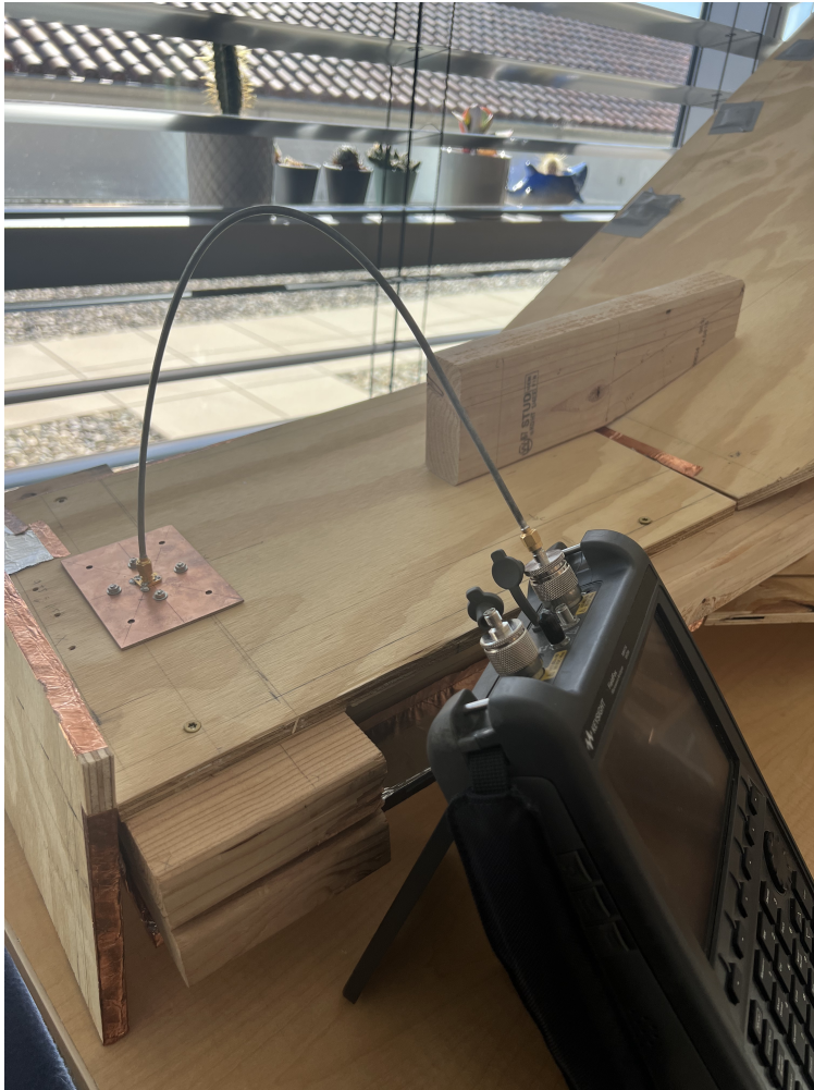
Figure 14: Horn antenna connected to Fieldfox Network Analyzer for impedance test.
