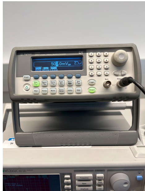
(b) Agilent 33220A Arbitrary Waveform Generator used to add a lower frequency FM deviation.
