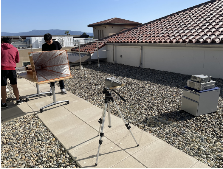
Figure 16: Directivity test set up, tape markings denote different angle measurement placement.
