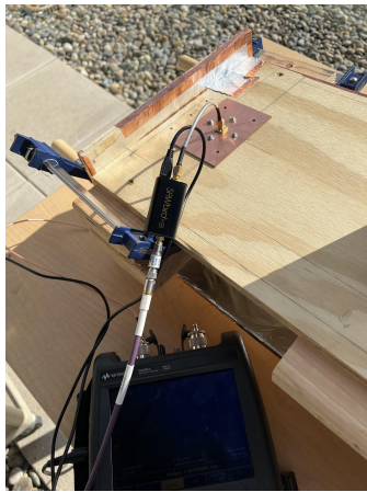
Coaxial feed to LNA input
