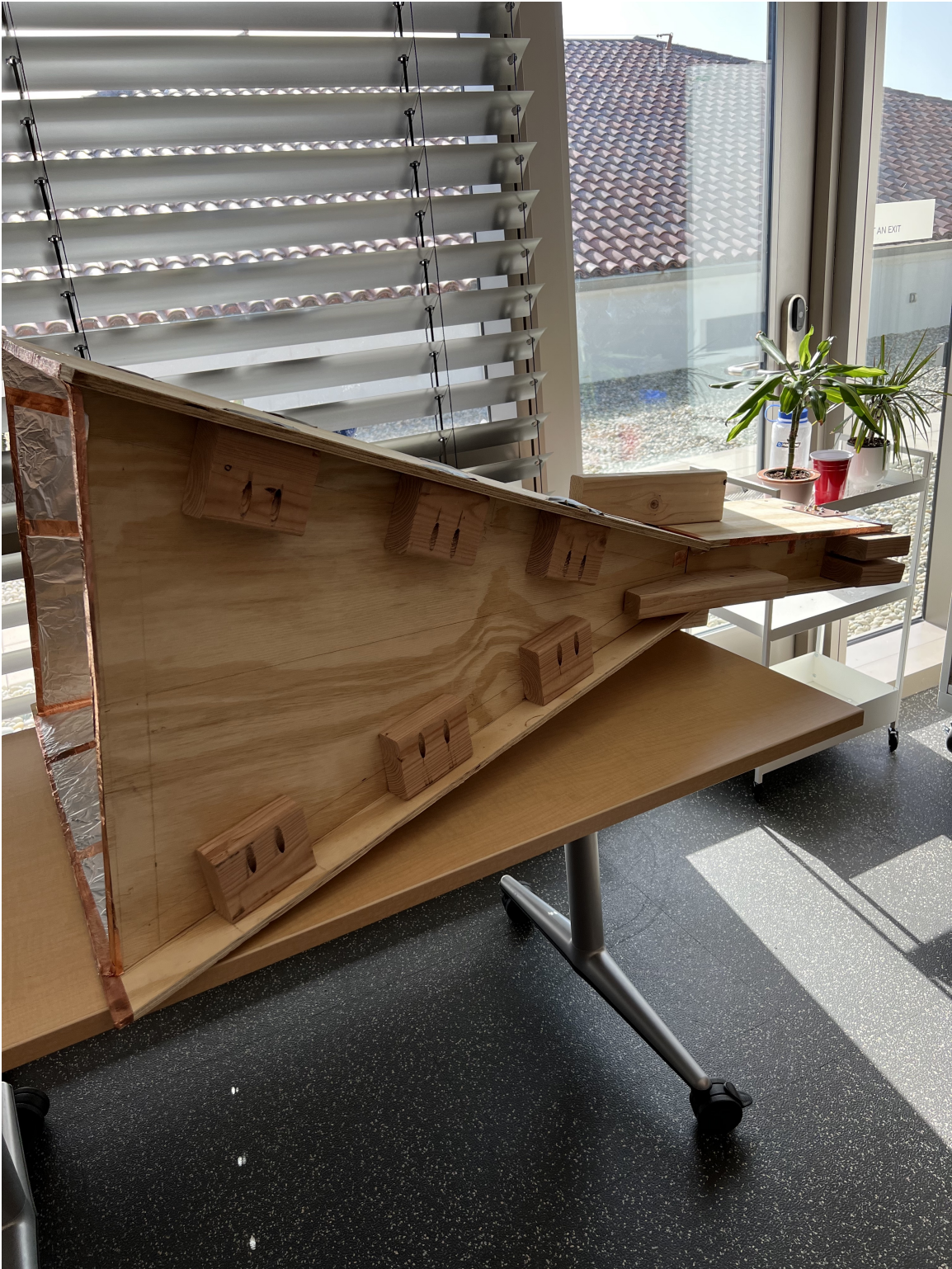
Figure 11: Completely constructed pyramidal horn antenna.
