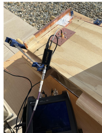
Coaxial feed to LNA input to Field Fox spectrum analyzer
