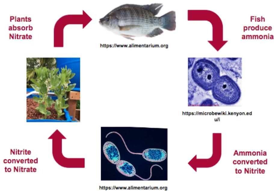
Figure 8: Nitrogen Cycle in an Aquaponic System.
