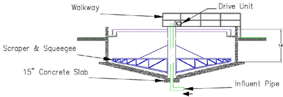
Figure 9: Section View of Secondary Clarifier.
