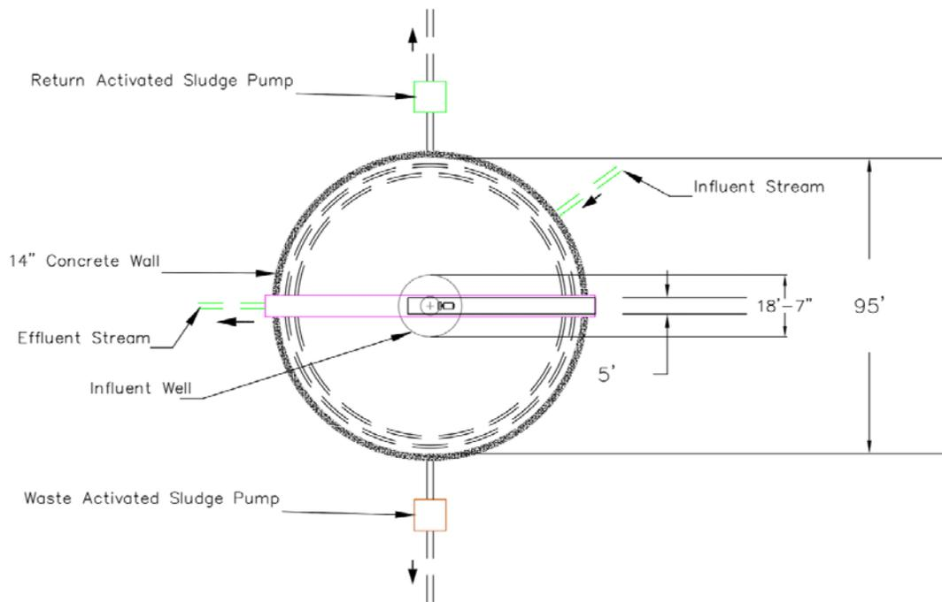
Figure 8: Plan View of Secondary Clarifier.
