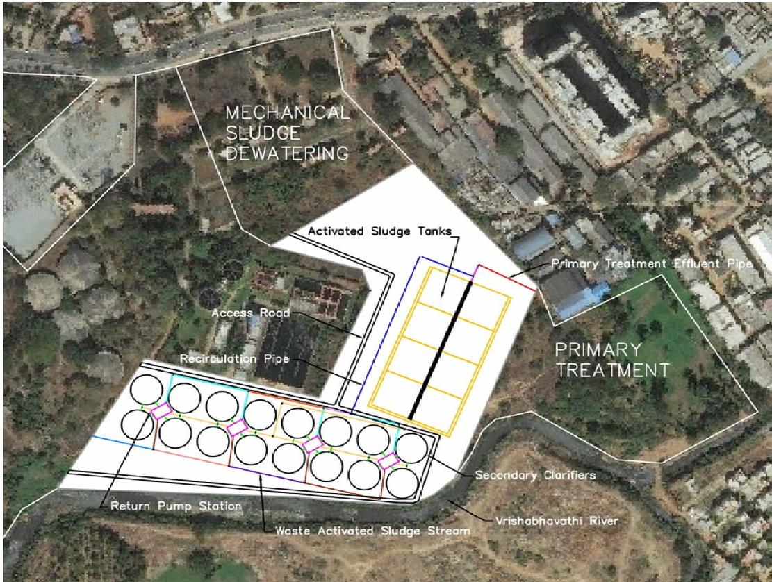
Figure 5: Site Layout & Secondary System Configuration.
