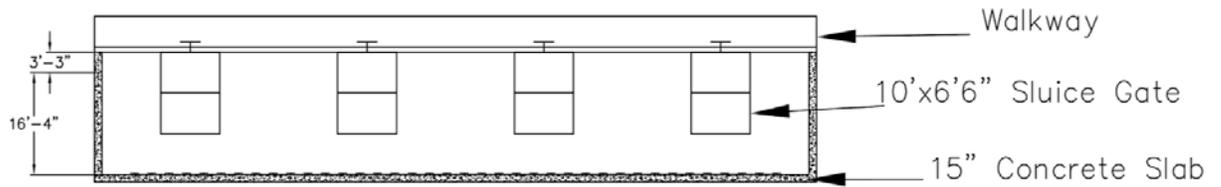
Figure 7: Section View of Activated Sludge Tank.
