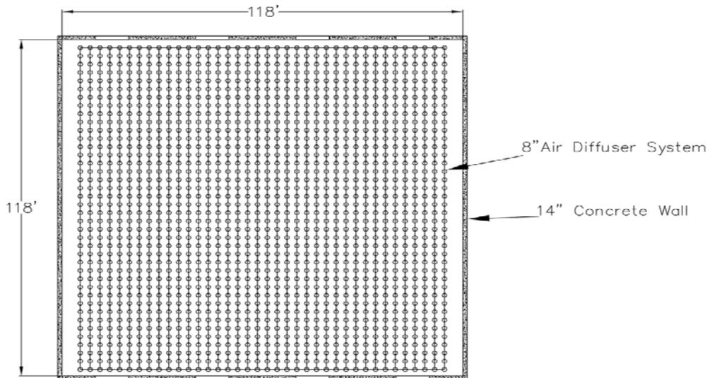
Figure 6: Plan View of Activated Sludge Tank.
