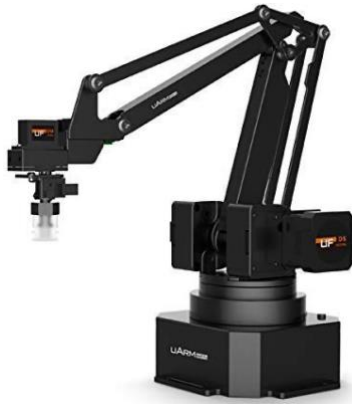
Figure 9: UArm Swift Pro with 4 DoF and Suction Cup
