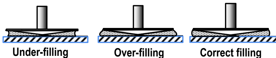
Proper loading of sample after closing the gap for cone and parallel plate geometry systems
