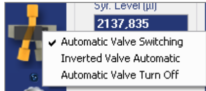
Figure 32 - Configuring Valve Automation
