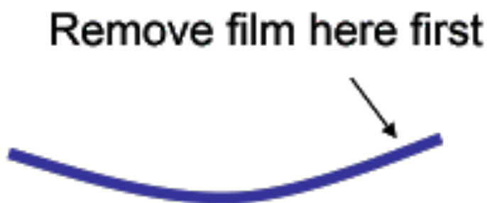
Figure 8. Demonstration of dry-film photoresist natural curl. Due to the difficulty removing the thin plastic film off of the photoresist film without damaging it, there is a need to standardize the approach to removing it that results in the smallest amount of damage possible.
