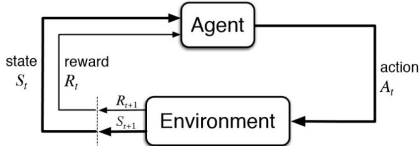
Figure 2: Reinforcement learning feedback loop
