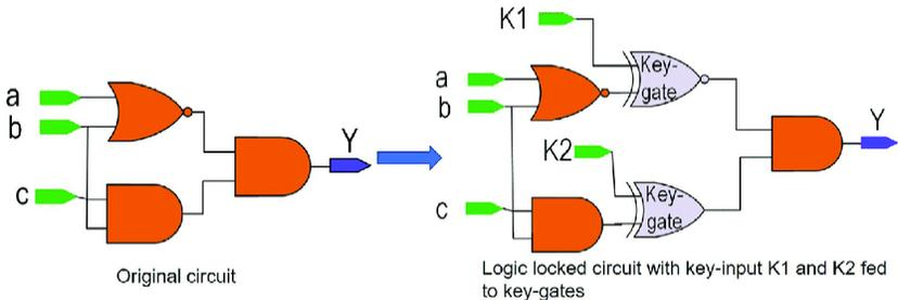
Figure 1: Logic Locking Example
