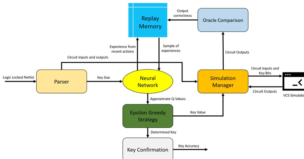
Figure 6: Block diagram of reinforcement learning attack
