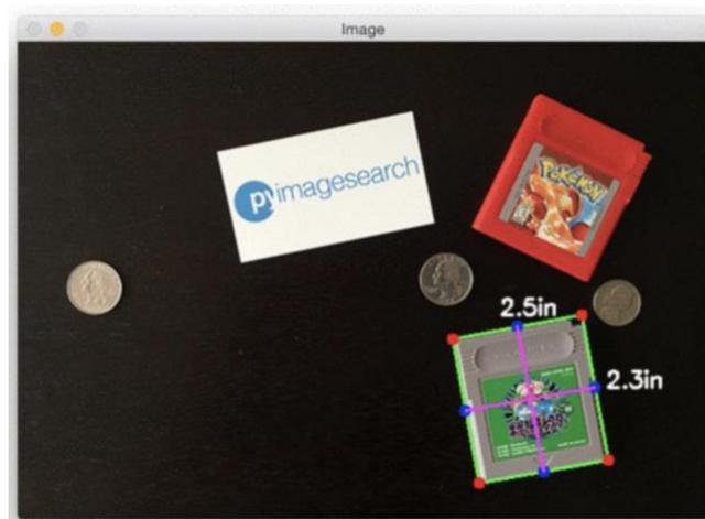
Figure 5 - Processed Image with Measured Object and Measurements Displayed [11]
