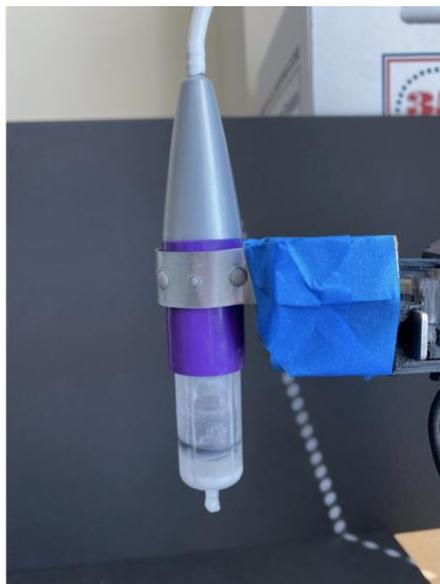
*Figure 13 - A side view of the extruder attached to the gripper*
