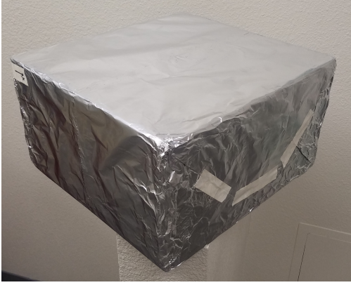
(a) Small rectangular prism cavity (19.6 cm x 35.5 cm x 32.6 cm).
