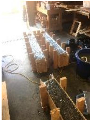
**Figure 10: Poured concrete beams sitting in the formwork.**
