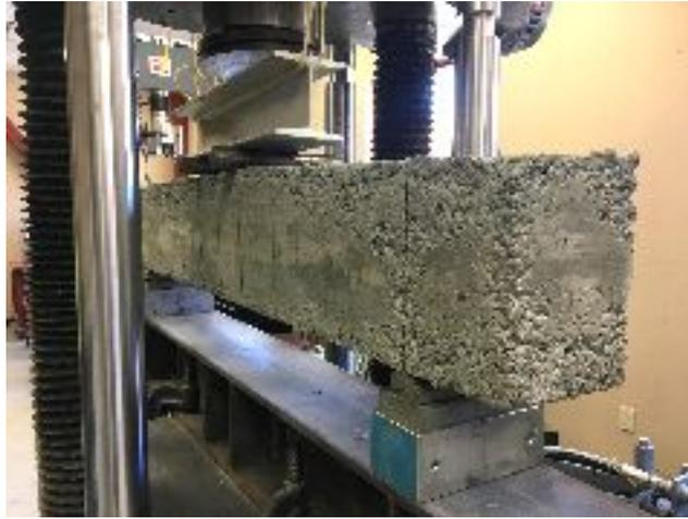
**Figure 11: Example of the testing apparatus for the full size beams.**
