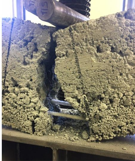
**Figure 12: Failed beam with fish netting reinforcement.**
