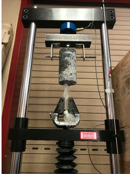
**Figure 14: Testing Apparatus for pull-out test using fish netting.**
