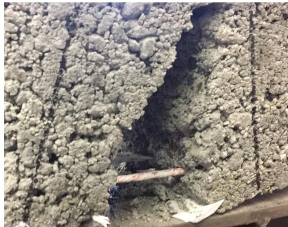
**Figure 13: Failed beam with grocery bag reinforcement.**
