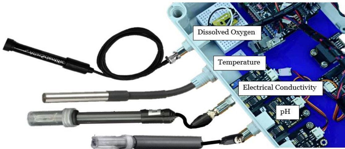
Figure 52. Visual representation of how the sensors will be connected to the Arduinos in the waterproof box
