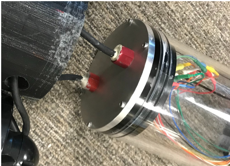
Figure A-3: Lateral Thruster Brace attached to Endcap Batteries Aft
