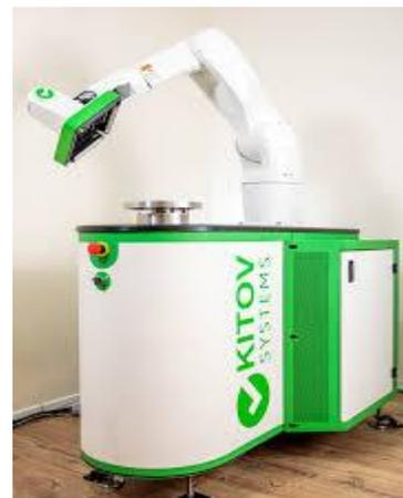
*Figure 2: Kitov System - Denso Robot w/ Camera [3]*
