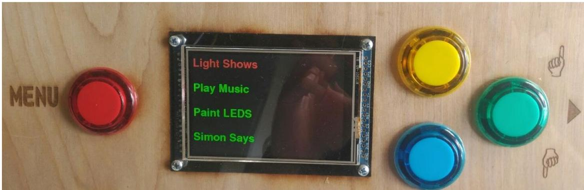
Figure 3.6: User Interface, TFT + Touchscreen and arcade buttons
