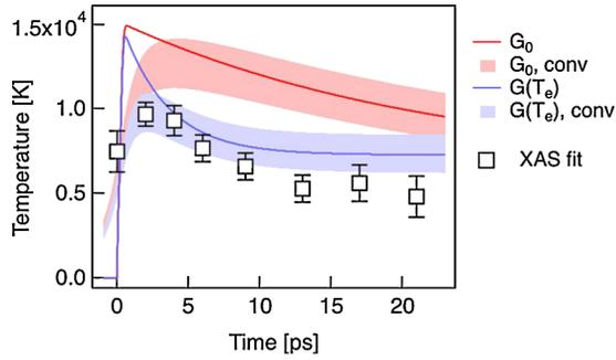
FIG. 4 (color online). The temporal evolution of the  $T_e$ . Experimental-derived values of the  $T_e$  are shown as squares. For  $G_0$  and  $G(T_e)$ , solid lines are the  $T_e$  calculated by the TTM. The shaded curves include the experimental accuracies in the  $E_d$  and the temporal resolution of the detector.
