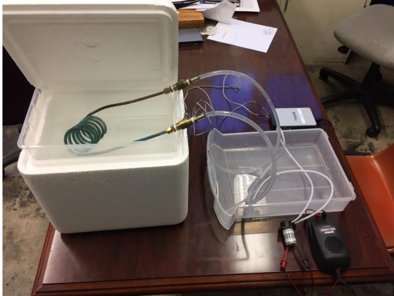
Figure 9: Experimental Heat Exchanger
