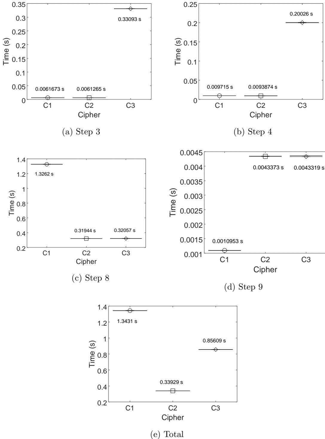
Figure 3.3: Processing time of various steps. This figure confirms that client verification of an ECDSA certificate requires about 5200% longer processing compared to RSA. In addition, signature verification using ECDSA is around 2000% longer than RSA. Furthermore, key exchange using DHE shows 300% longer processing time than using ECDHE. In general, the processing overhead of C1 and C3 are 300% and 150% higher than C2, respectively.
