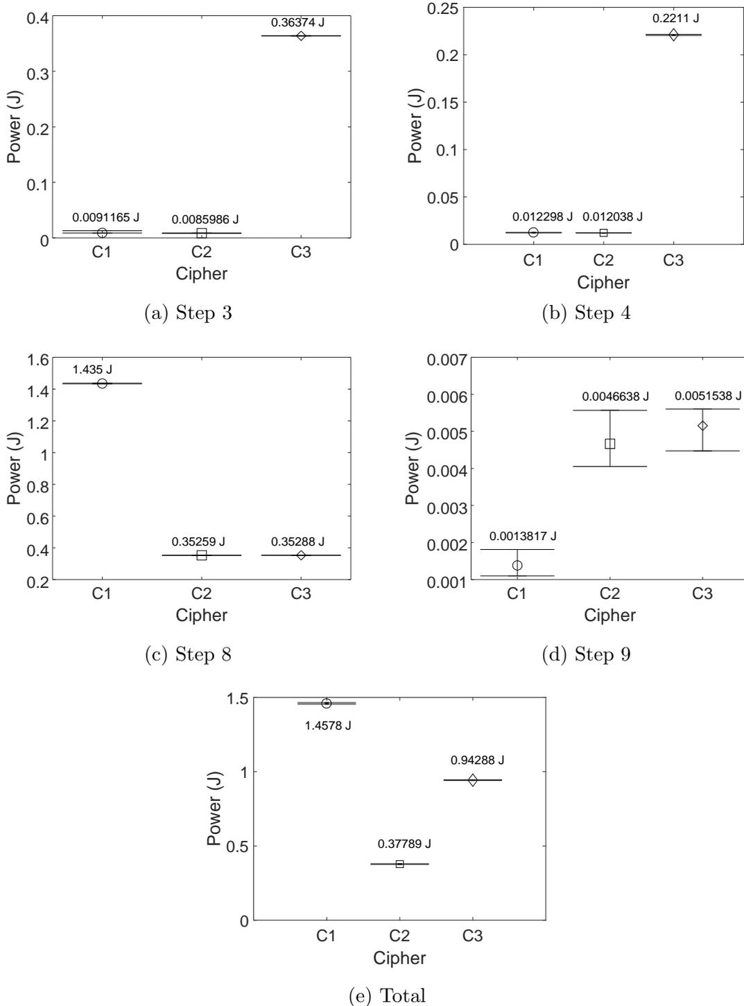
Figure 3.4: This figure confirms that client verification of an ECDSA certificate requires about 3900% more energy compared to RSA. In addition, signature verification using ECDSA requires around 1700% more energy versus RSA. Furthermore, key exchange using DHE shows 300% more energy compared with ECDHE. In general, the processing overhead of C1 and C3 are 300% and 150% higher than C2, respectively.
