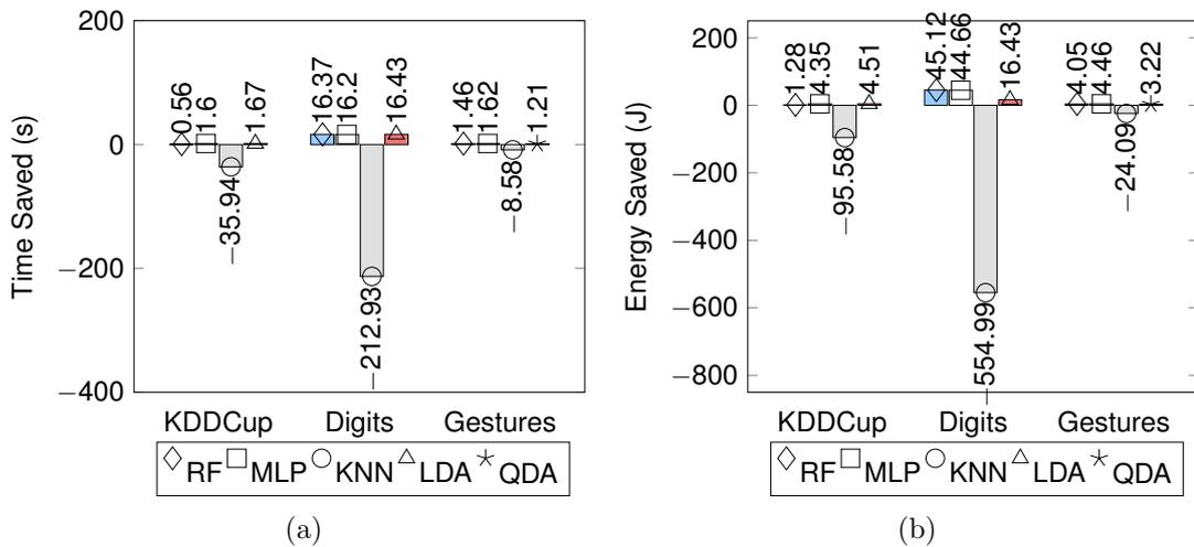
Figure 4.5: RF, MLP, and LDA all demonstrate overhead savings when applied to data before transmission; most notably, RF applied to the Digits dataset saves 45.119 J and 16.37 seconds per 2000 image buffer. KNN is a poor choice for real-time anomaly detection scenarios given that it causes net time and energy loss across all datasets.
