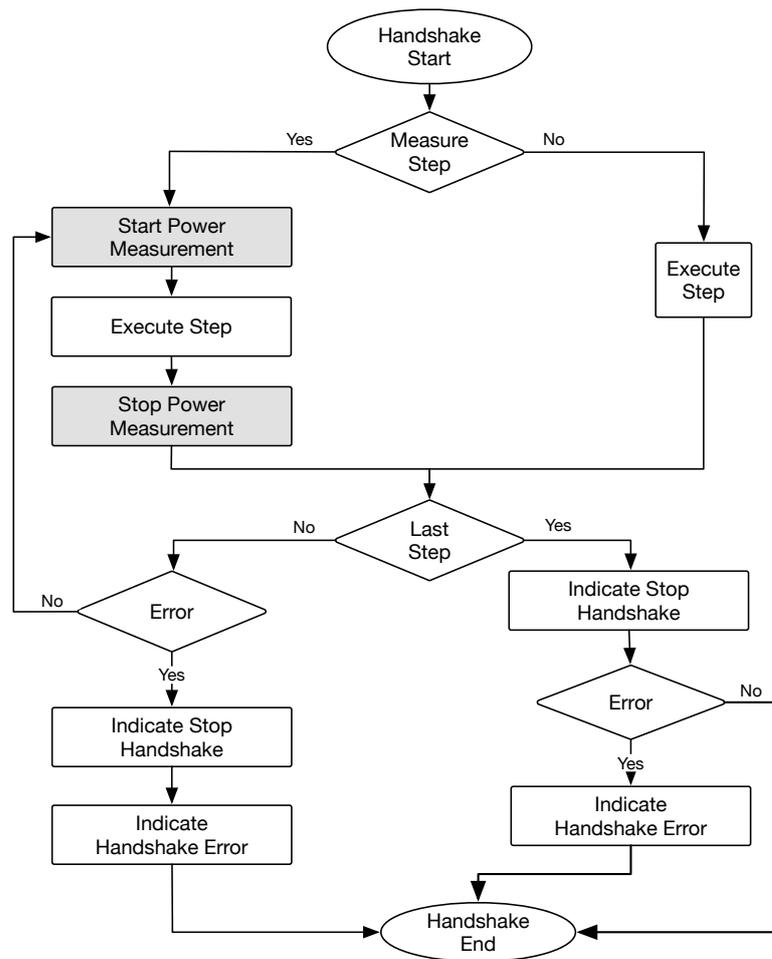
Figure 3.2: The flow diagram of measurement methodology.
