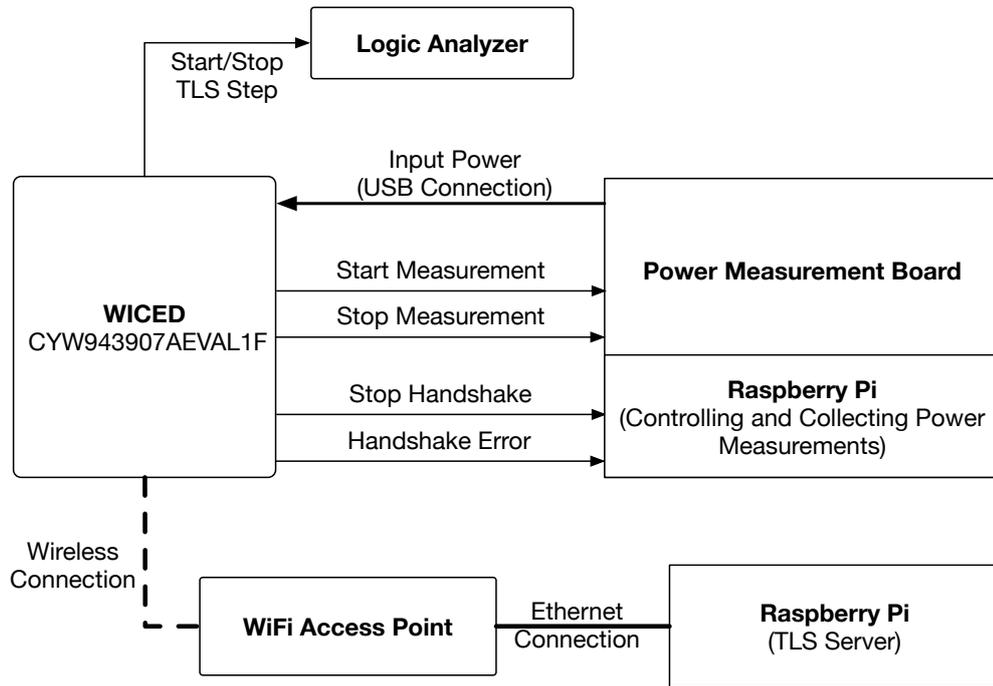
Figure 3.1: The components and interconnection of the testbed used.
