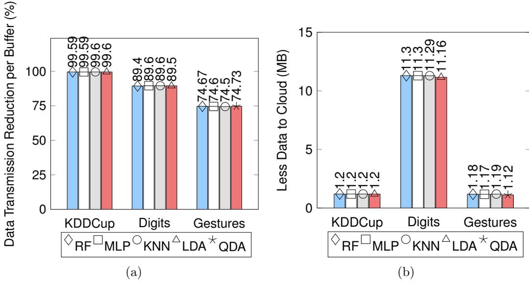
Figure 4.6: From (a) we observe that the models reduce approximately 90% of the observations sent from Digits’ buffers, 76% of the observations sent from Gestures’ buffers, and 99.5% of the observations sent from KDDCup’s buffers. The resulting saved cloud storage shown in (b) is substantial, especially for Digits dataset where we saved nearly 12 MB of data sent per 2000 image buffer.
