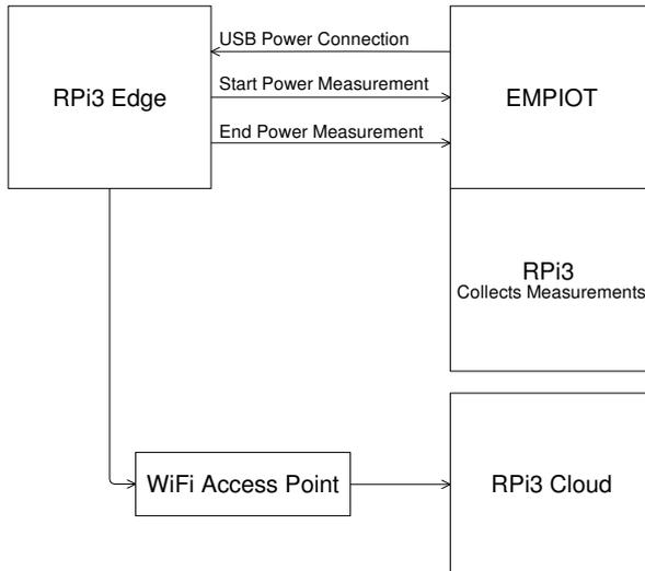
Figure 4.1: The testbed used for our experiment inclusive of three RPi3s and the EMPIOT energy measurement platform. The RPi3 hosting EMPIOT captures energy measurements of the edge RPi3 transmitting data to the cloud RPi3.
