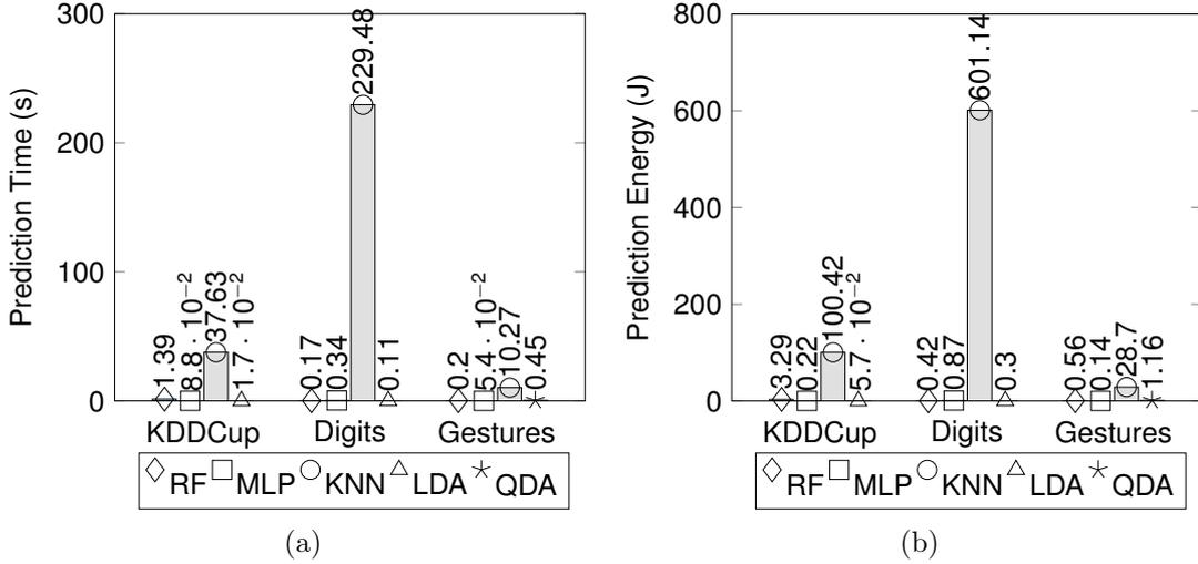
Figure 4.4: LDA offers the most cost-effective prediction phase for both Digits as well as KDDCup datasets as shown in (a) and (b). MLP offers the most cost-effective prediction phase for the 64 feature Gestures dataset. KNN costs nearly 600% more energy and 650% more time than the next best performing model across all datasets.
