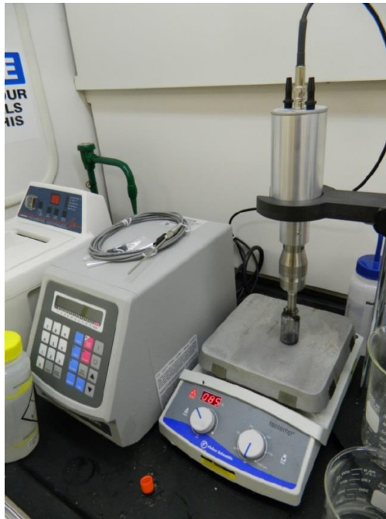
Fig. 3.1 Photograph of stock ultrasonication procedure. The ultrasonicator probe is inserted into a vial of unmixed nanofluid stock placed on a hot plate.
