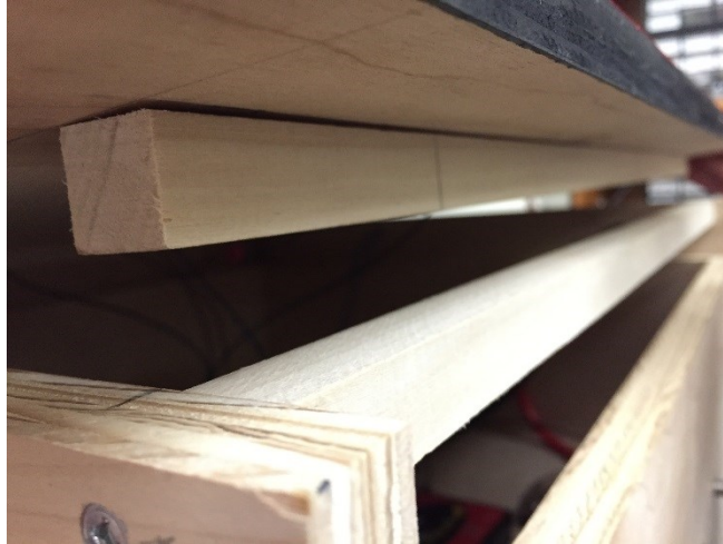
Figure 3.6: Docking station platform alignment bars
