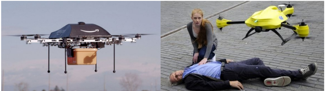
Figure 1.1: Left: Prototype drone for Amazon’s planned Prime Air delivery service. Photo courtesy of amazon.com. Right: Conceptual defibrillator-equipped drone developed by Delft University of Technology. Photo courtesy of tudelft.nl.
