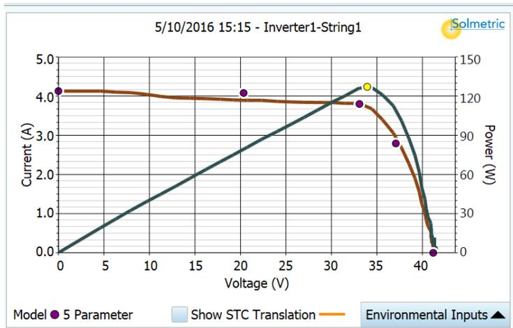
Figure 27: IV Curve Collected by Solmetric Analyzer
