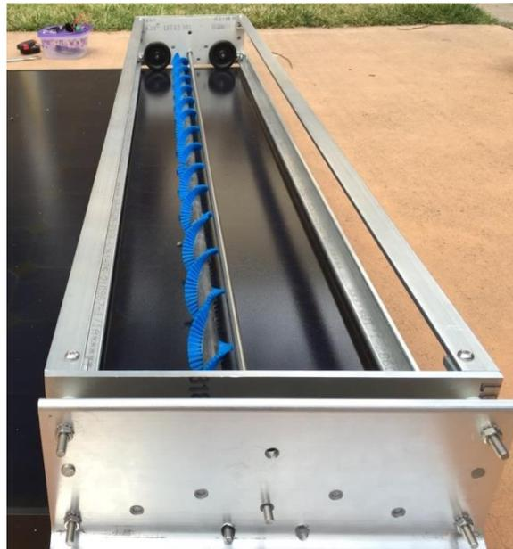
*Figure 14: Driveshaft (right of brushes) transfers power across system*
