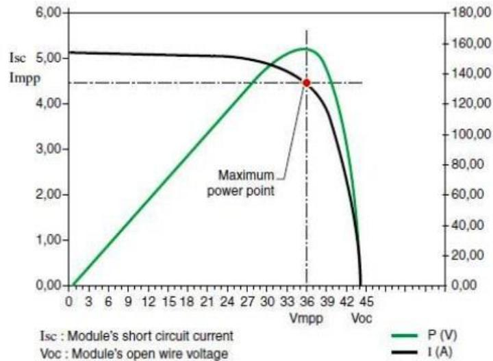
Figure 26: Typical IV Curve of a Solar Panel Showing MPP
