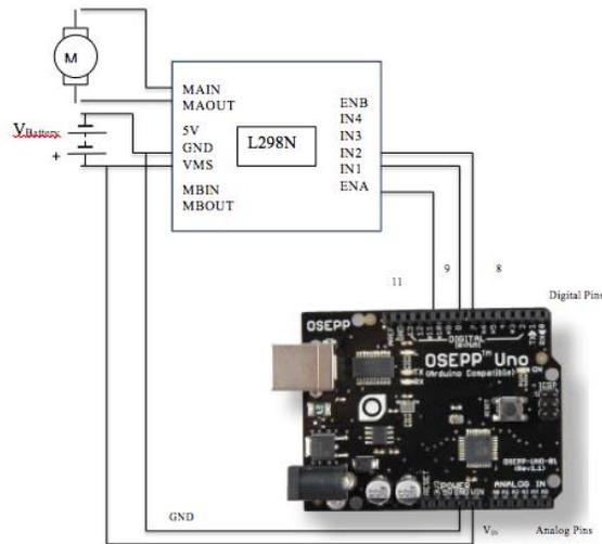
Figure 21: Diagram of the Interconnections Between the Control System Components
