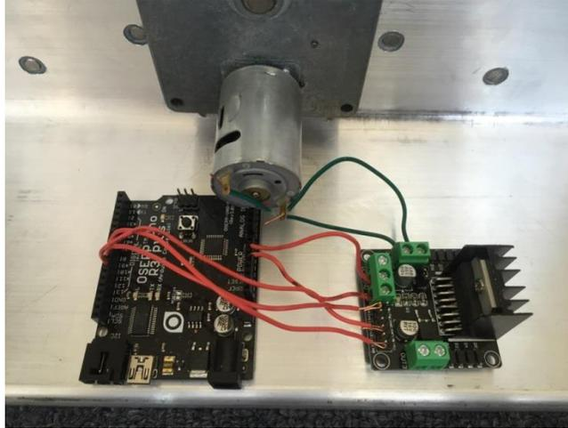
*Figure 20: Control system hardware overview*
