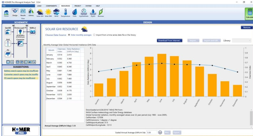
Figure 35: Homer model architecture and annual global horizontal irradiance used for simulation<sup>9</sup>
