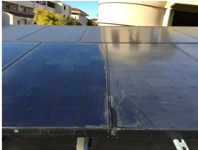
*Figure 1: Cleaned panel (left) vs. Soiled panel (right) (Team Photo)*
