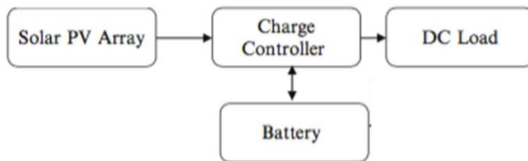
*Figure 23: Flowchart of Stand-Alone PV System<sup>7</sup>*
