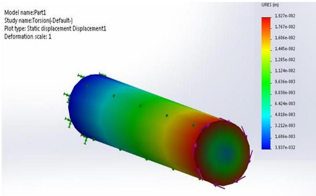
Figure 17: Solidworks FE driveshaft displacement analysis
