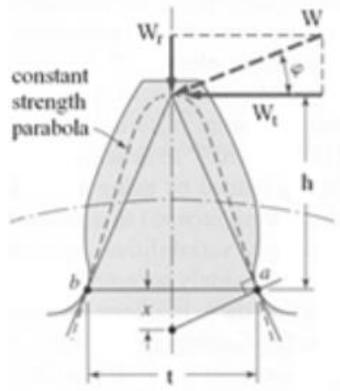
Figure 18: A Free Body Diagram of a Gear Tooth<sup>6</sup>
