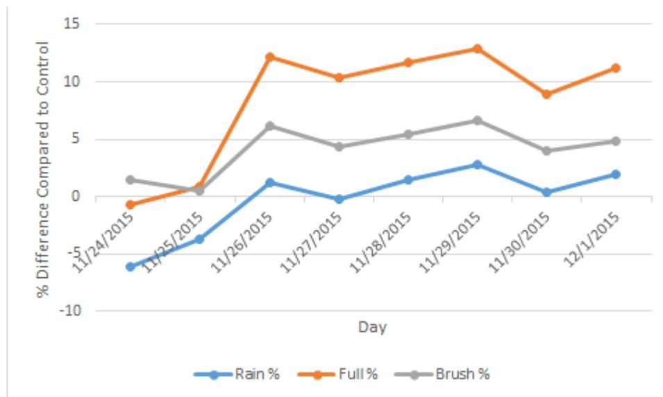
Figure 13: Improvement in Solar Energy Generation after Cleaning (App. G-1)
