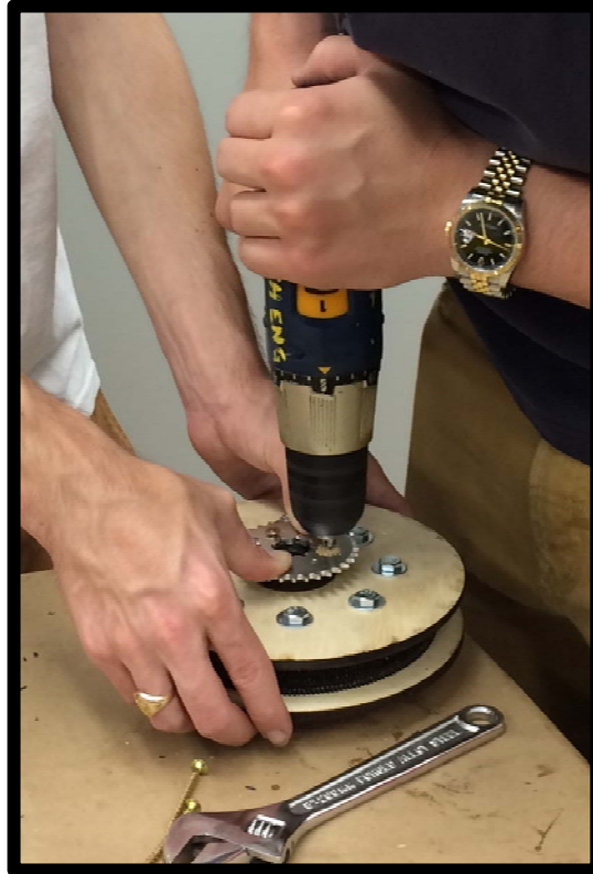
Figure 15: Iteration 1.2 Wheel being fitted with custom sprocket
