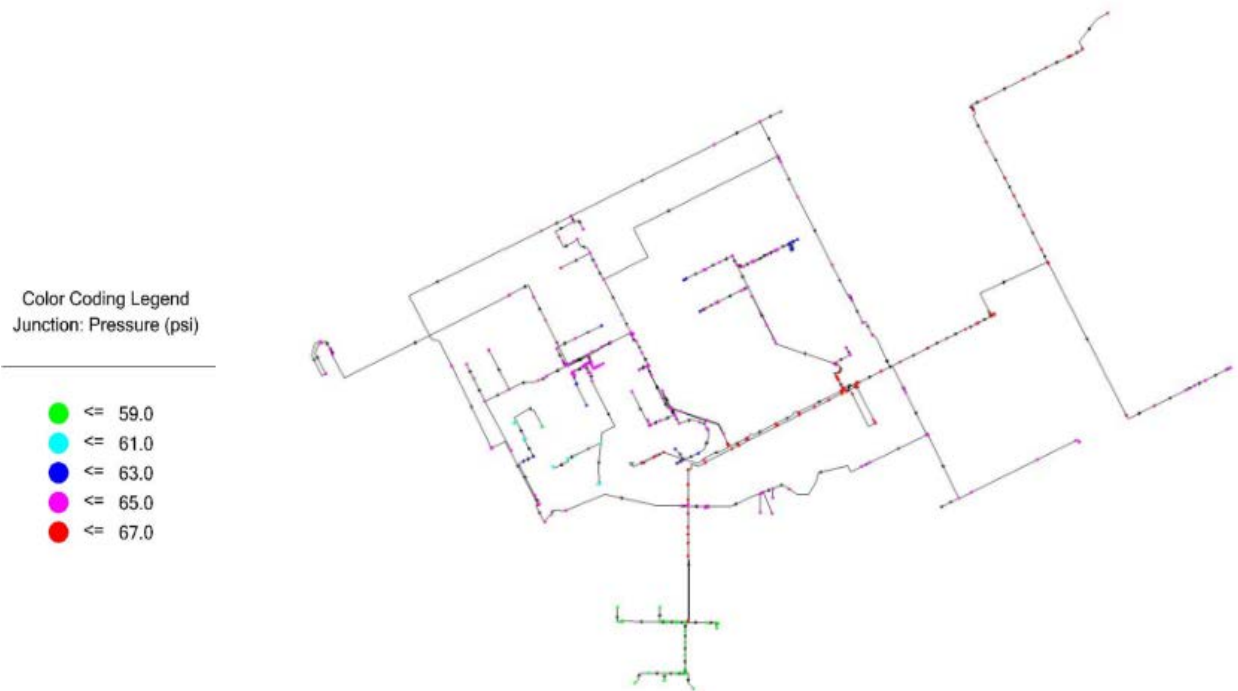
Figure 24: 2W PVC & steel pressure readings during peak operating hours
