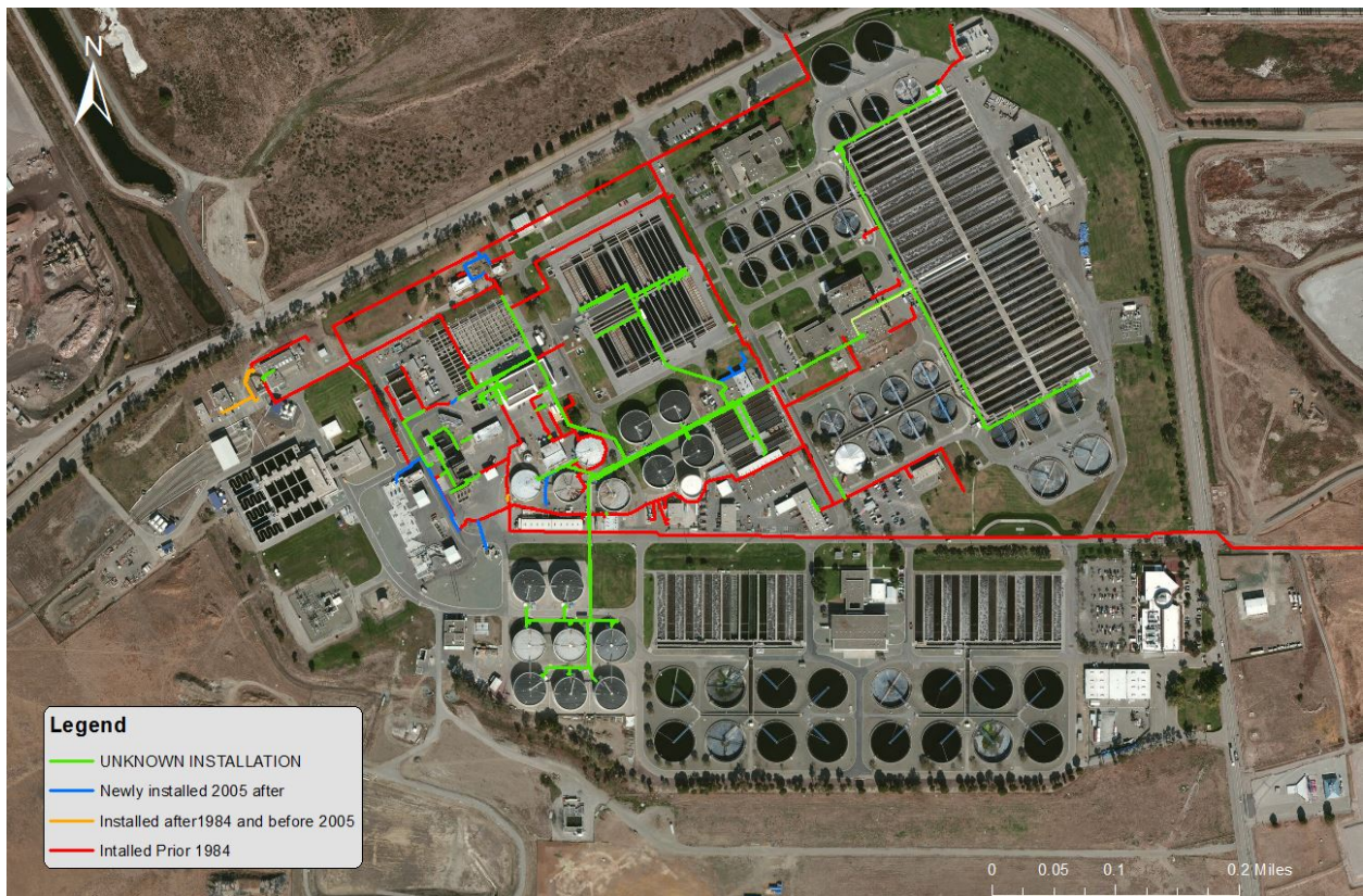
Figure 9: 2W ArcMap projection of pipe age color-coded by year of pipe installation
