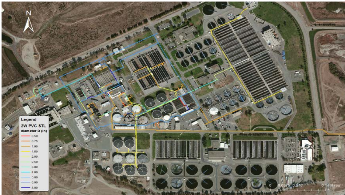
Figure 26: ArcMap rendition of the 2W system with color coding depicting looped pattern
