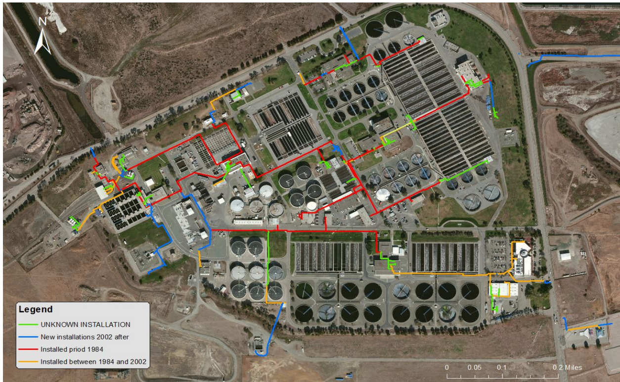
Figure 8: 1W ArcMap projection of pipe age color-coded by year of pipe installation
