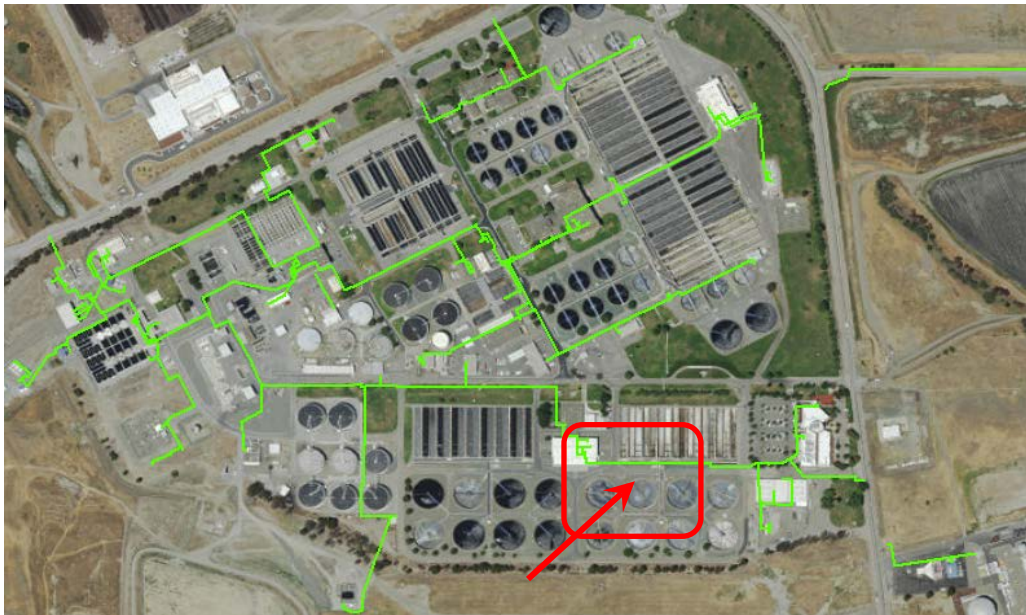
Figure 28: Aerial rendition of the 1W system connection to the Environmental Services Building
