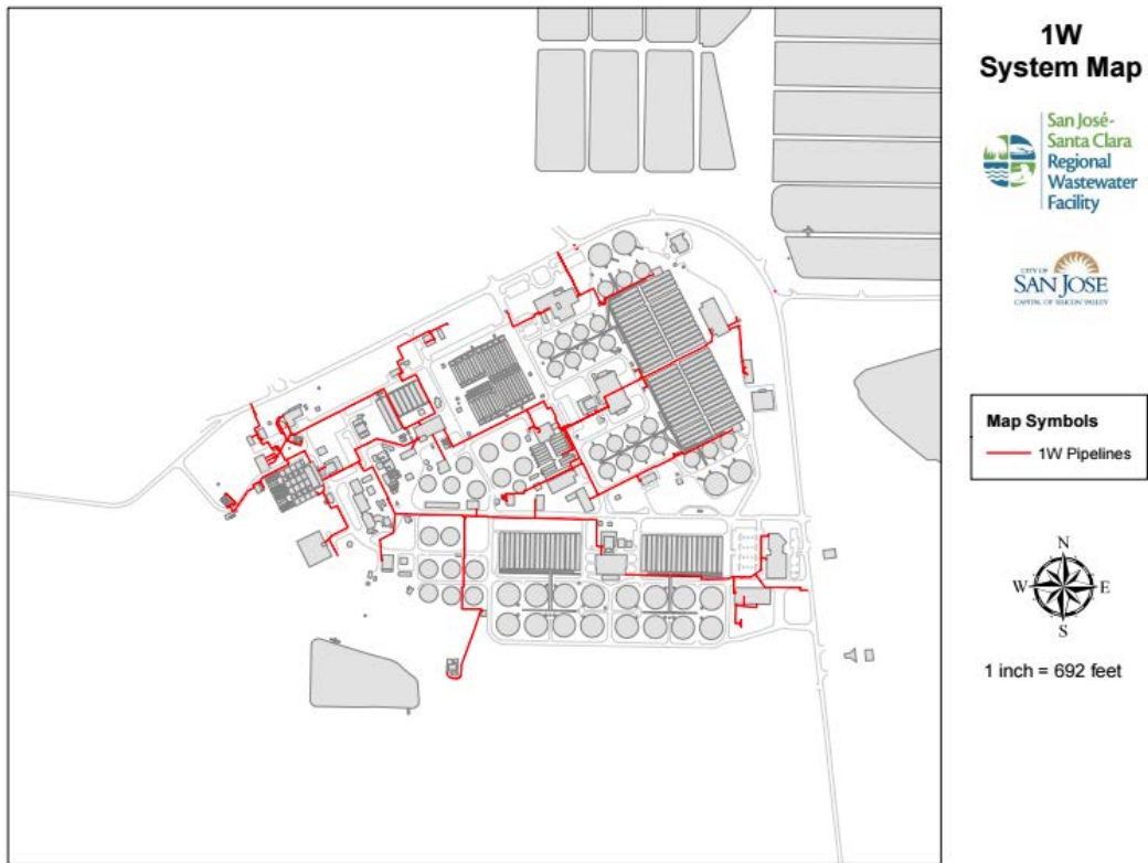
Figure 5: 1W Existing System Aerial Layout
