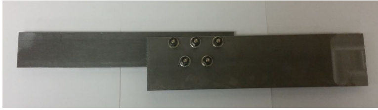
Fig. 13: Bolt test assembly used in this experiment.
