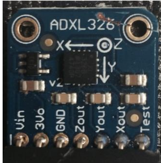
Figure 10: ADXL 326 Gyroscope and Accelerometer Module
