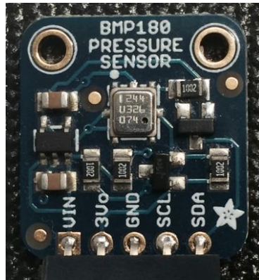
Figure 8: BMP180 Pressure and Temperature Sensor Peripheral.
