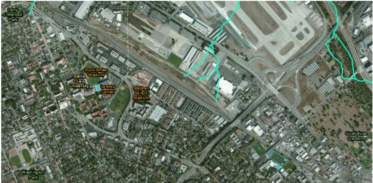
Figure 5 - Map of present city of Santa Clara overlaid with previously known historical channels. [Map generated in Arc GIS 10.1, data courtesy of SFEI 2011, provided by ESRI]
