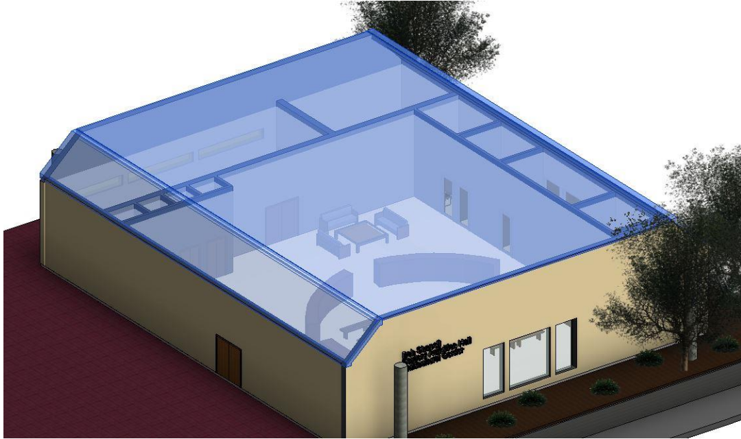
Figure 21. A 3D capture of the renovated MCC, highlighting the metal deck roof.
