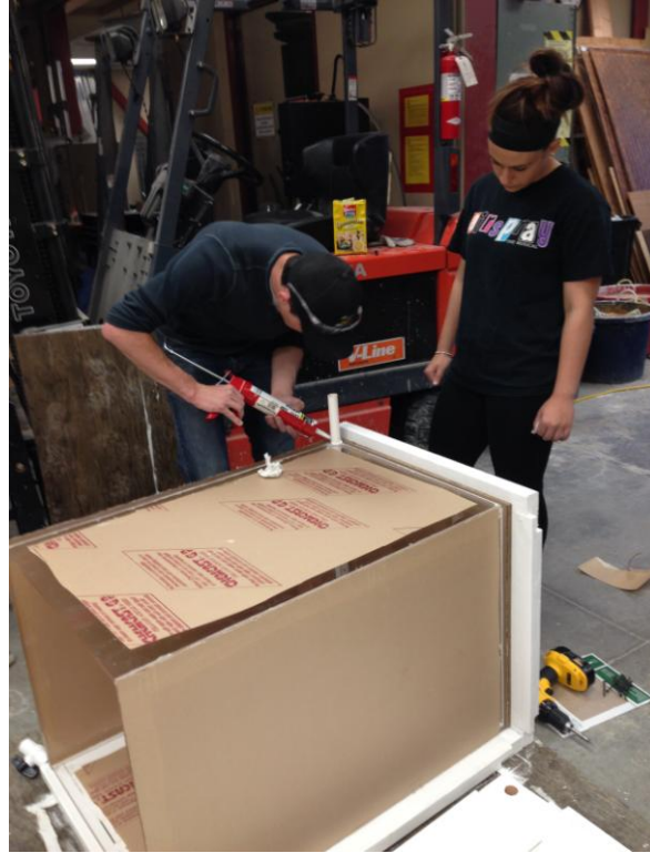
Figure 19: Caulking around the PVC pipe outlet prevented leaking
