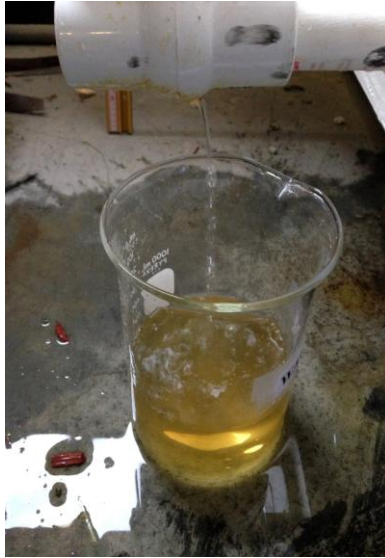
Figure 28: Discharge water tainted with mulch dye
