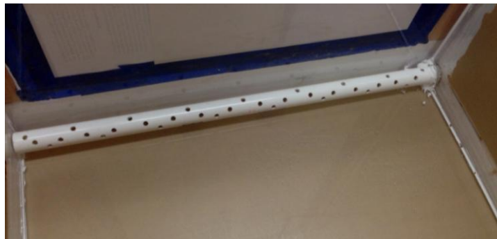
Figure 18: Perforated PVC pipe to collect drainage water from the model
