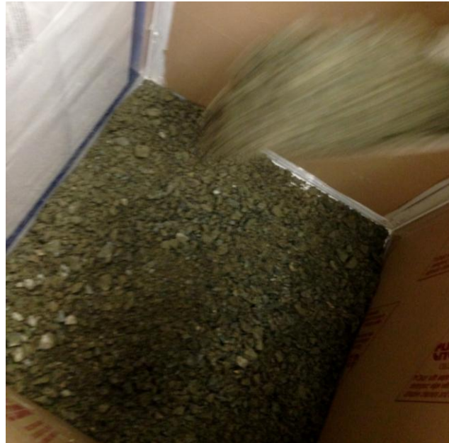
Figure 20: Filling the model with the Class 2 Permeable Gravel layer
