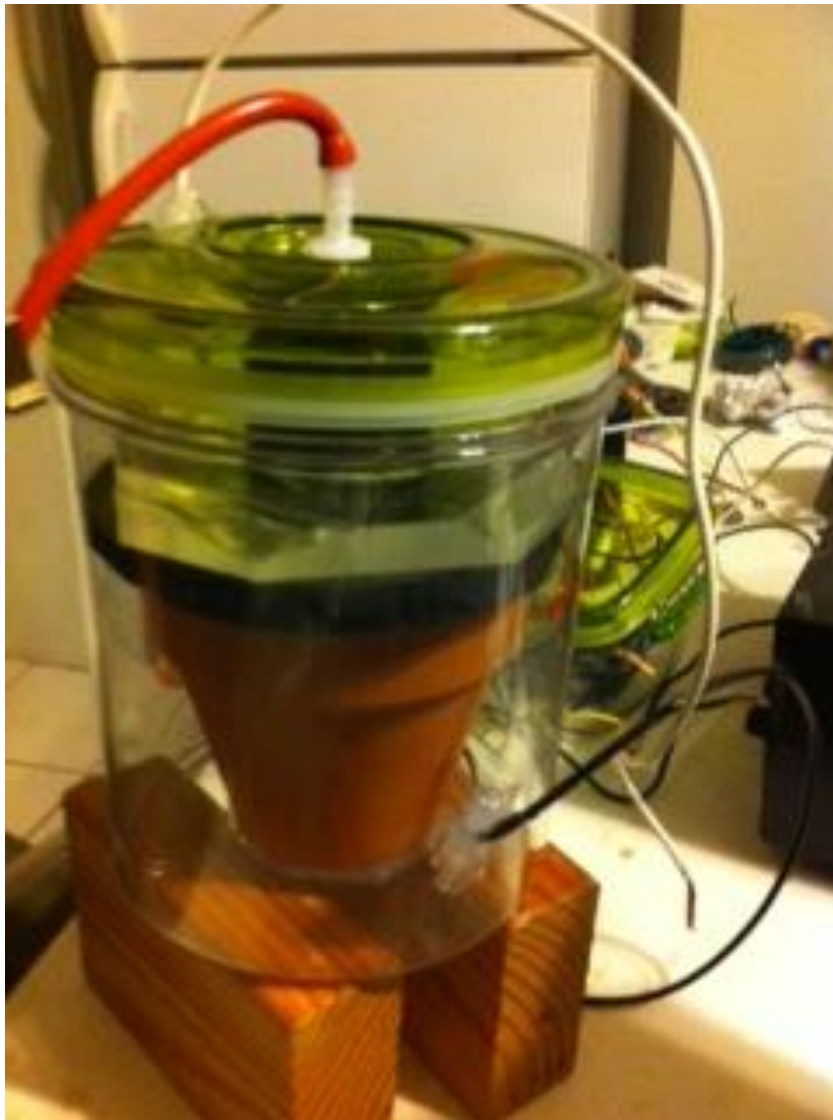
Figure 4: Development of third prototype with ceramic pot, sealable container, and gas switches.
