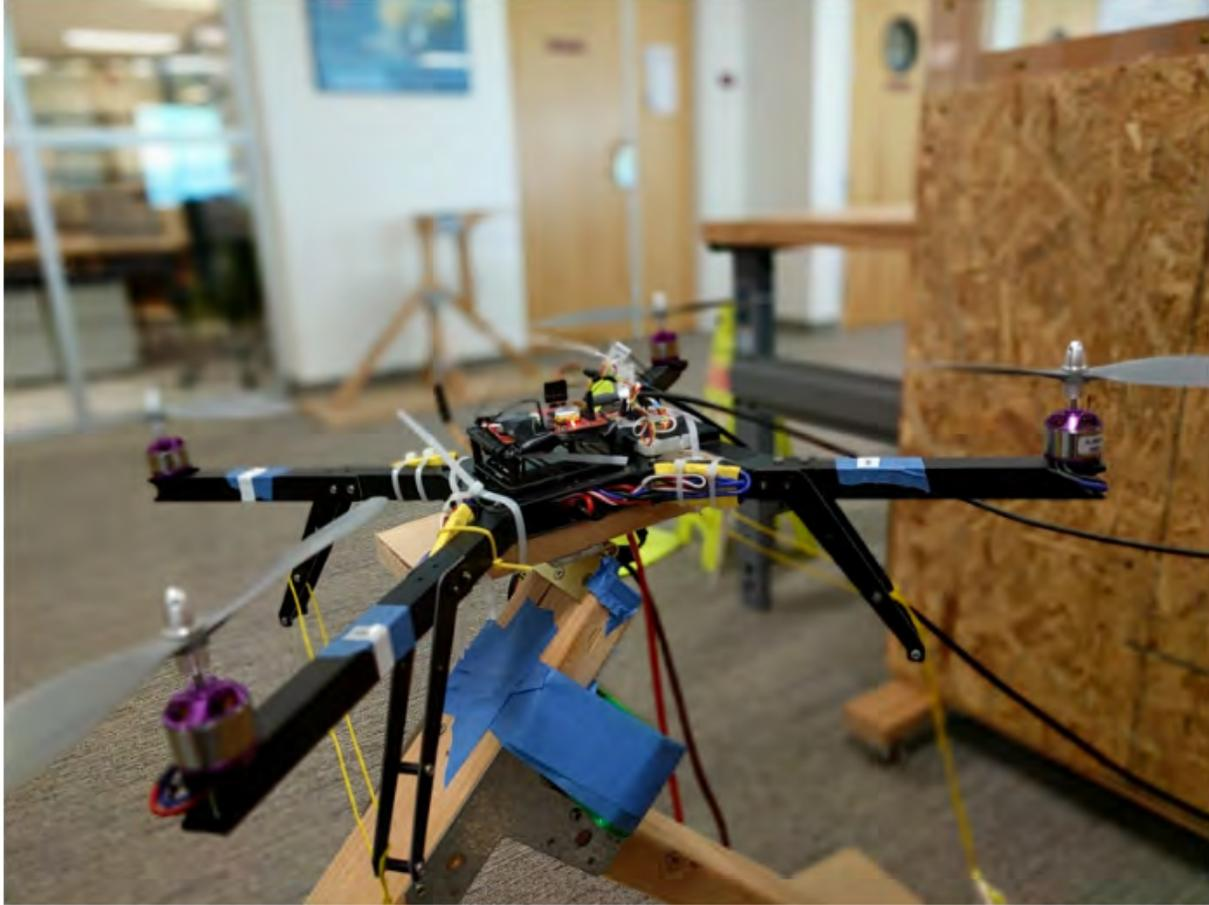
Figure 1.1: UAV Development Drone
