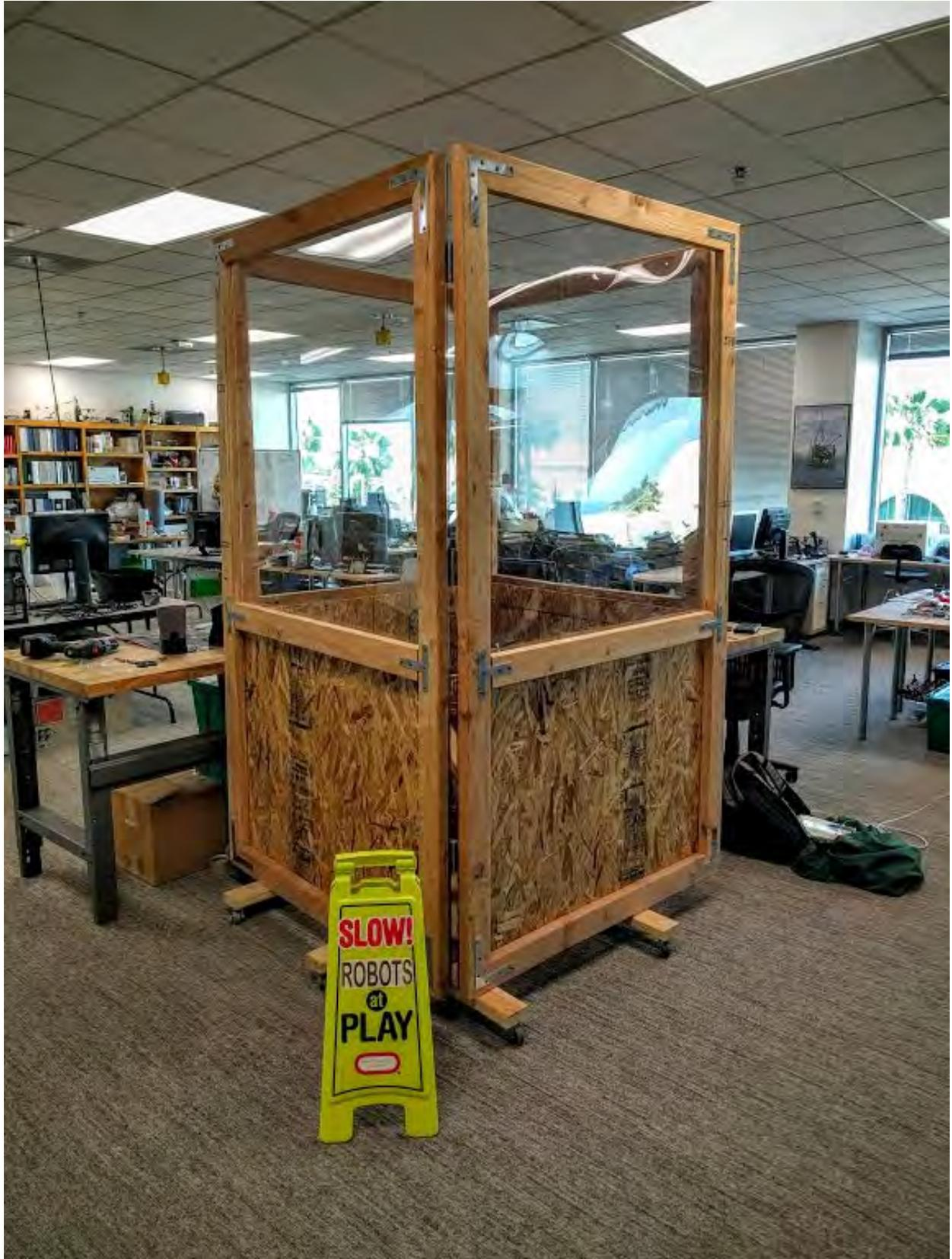
Figure 2.4: Drone Development Cage
