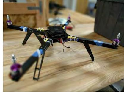
Figure 1: Frame of the drone
