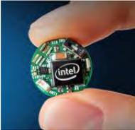
Figure 2: Intel Curie Processor
