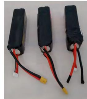
In both photos, the batteries on the left appear to be in good condition; the cells still need to be checked to make sure that the battery is balanced. The middle batteries are started to bloat and should be disposed of and no longer used. The batteries on the right have physical damage and should also be disposed of.
