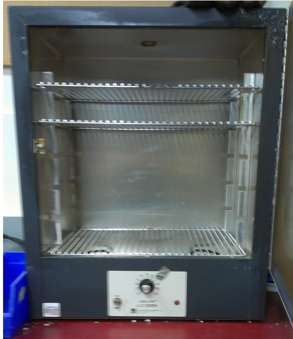
Figure 9.4: Oven used for thermal cycling.
