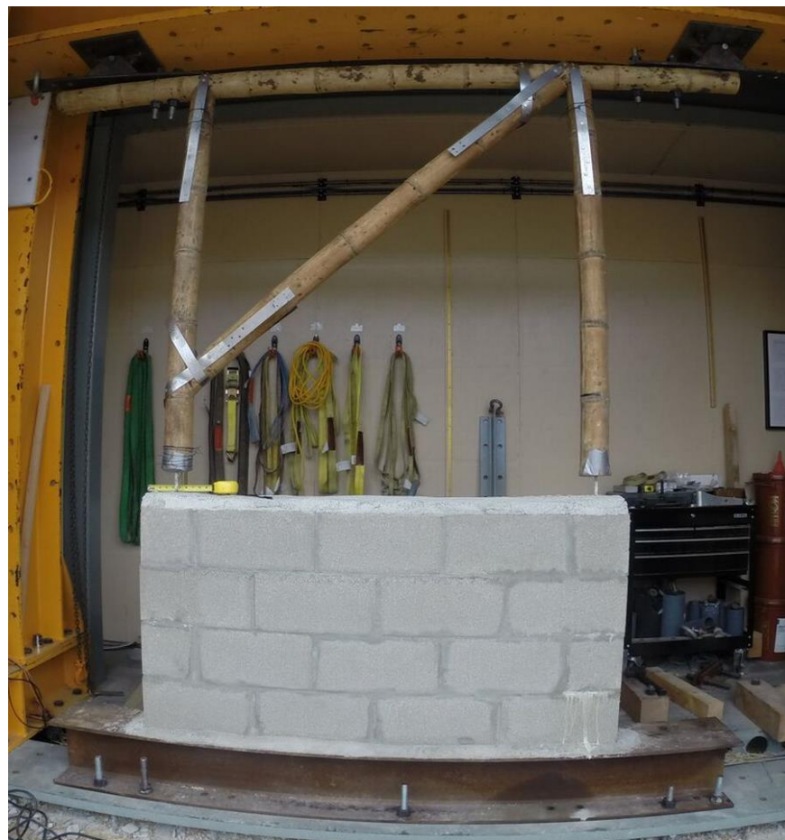
Figure 23: Full-Scale Wall Specimen after frame connection modifications
