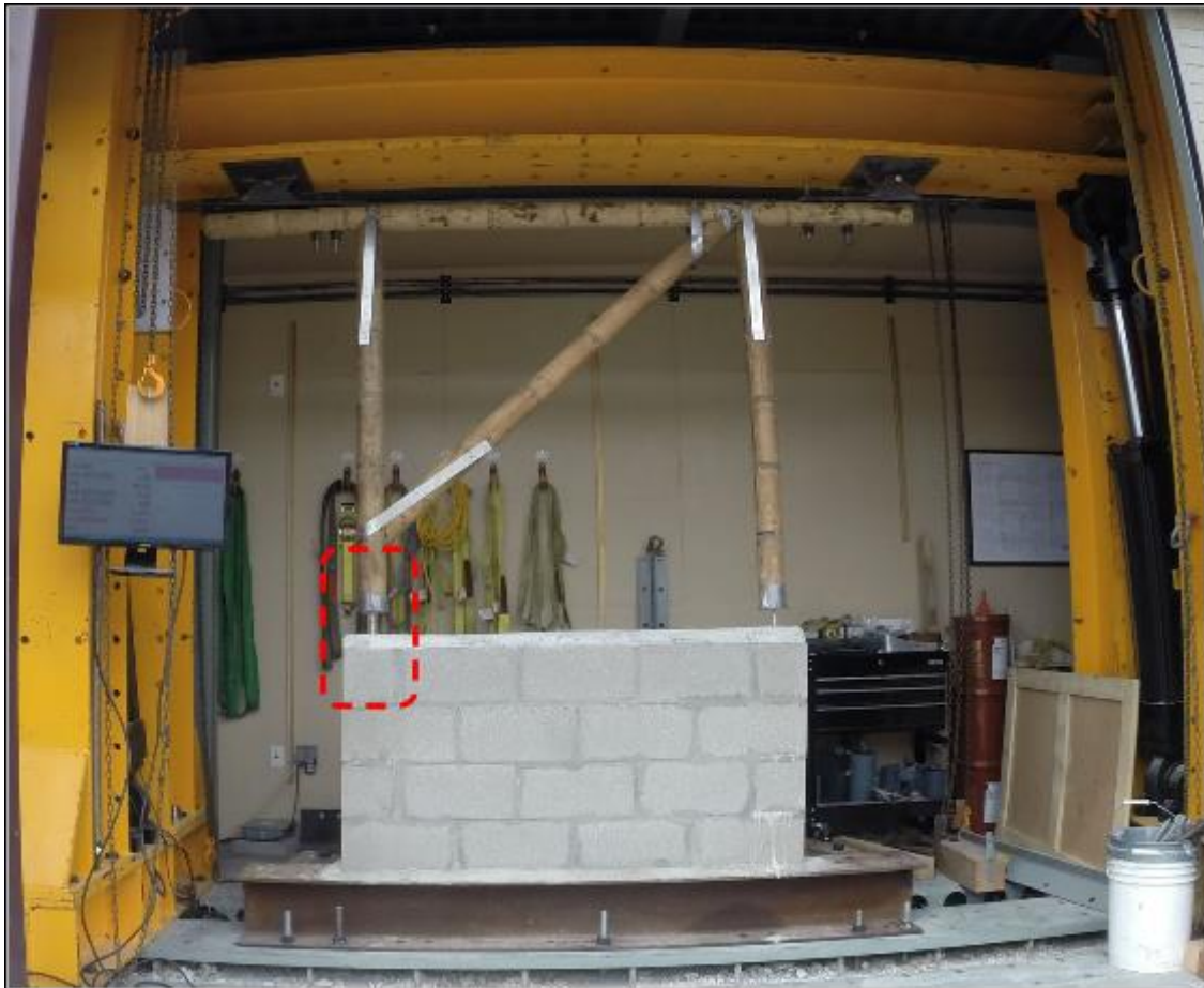
Figure 21: Full-Scale Wall Specimen in seismic simulator machine with ductile hinge mechanism boxed in red
