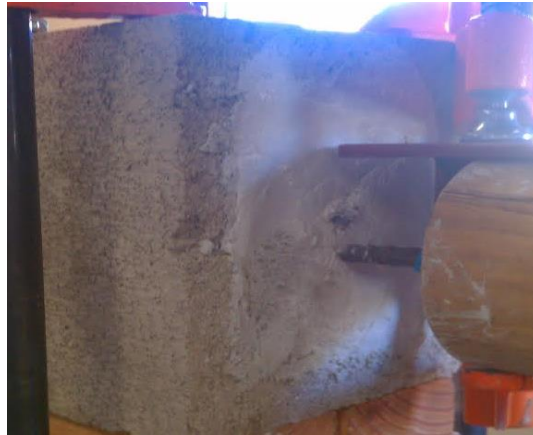
Figure 14: Isolated Unit Specimen 4 after testing demonstrating rebar dowel rupture
