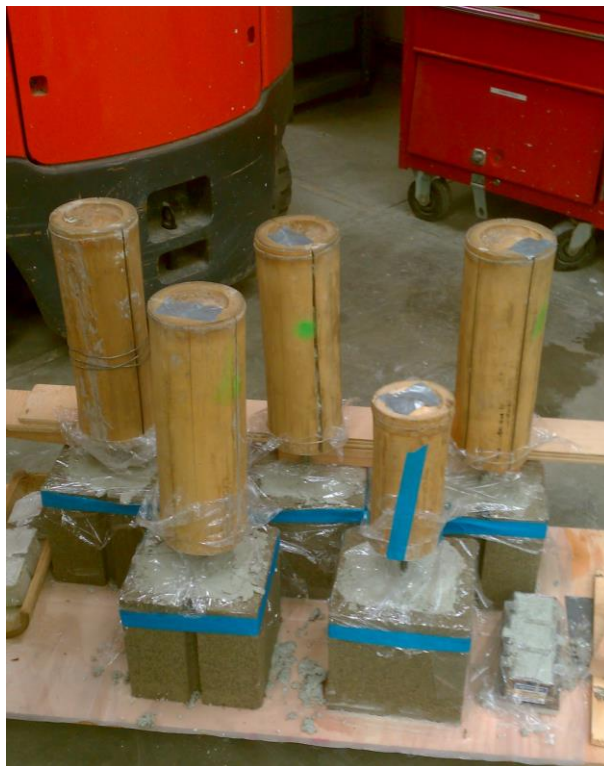
Figure 6: Isolated unit specimens in curing process
