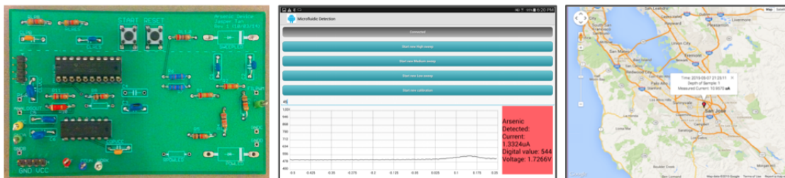
Figure 1.4: AquaSift's potentiostat device, Android application, and online database (L-R)
