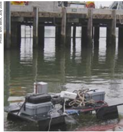
Student-designed autonomous surface craft uses multibeam sonar for bathymetric mapping of Moss Landing, Calif.
