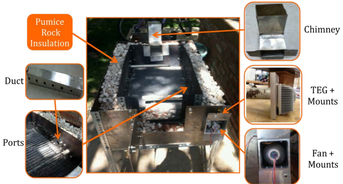
Figure 2. The key features of the stove body, ventilation system and power generation system.
