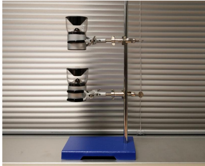
Fig. 2.16: Vertical configuration for catadioptric stereoscopy
