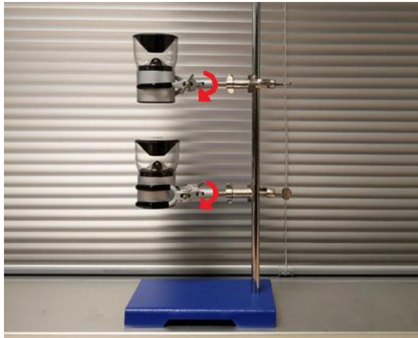
Fig 3.6: Primary sources of non-rigidity in the position adjustment system
