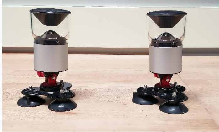
Fig. 2.14: Horizontal configuration for catadioptric stereoscopy
